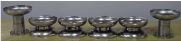
Figure 4: Dumbbells and 5-cell Nb cavity
