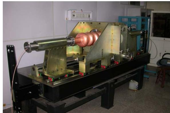
Figure 3: Tuning System for Multi-cell Cavities.
