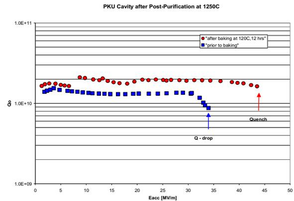
Figure 5:  $Q_0$  vs.  $E_{acc}$  of the single cell large grain cavity.
