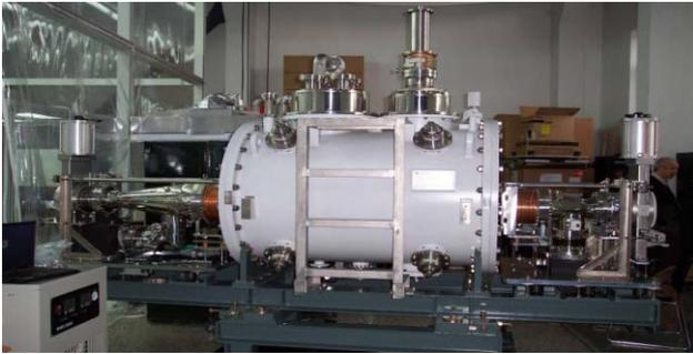
Figure 7a: 500 MHz cavity assembled at KEK.
