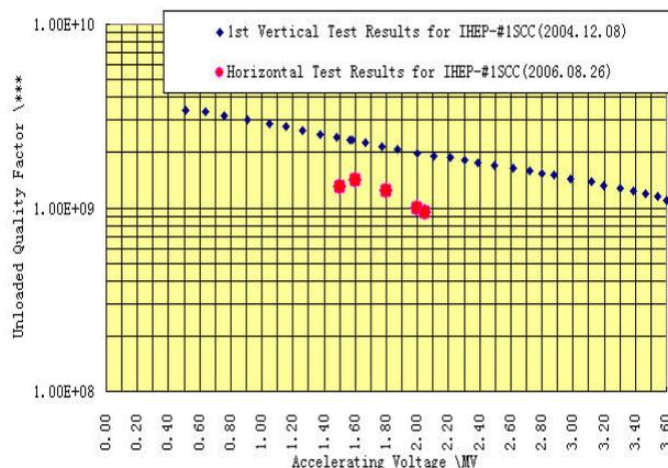
Figure 7b: Vertical and Horizontal test results at IHEP
