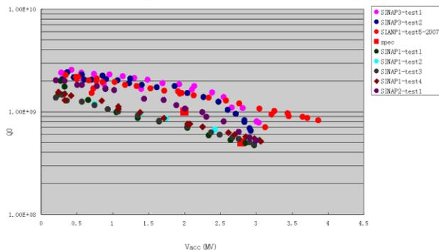
Fig.9 Vertical test results of SIAP single cell cavities
