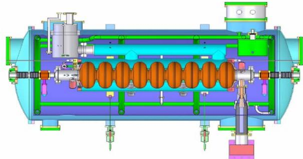
Figure 2: Layout of PKU Superconducting Accelerating Module.
