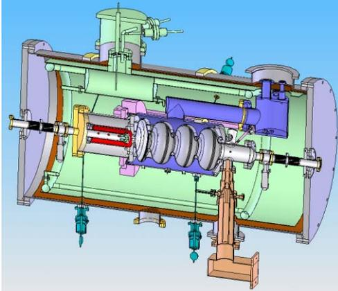
Figure 1: Layout of DC-SC Photo-injector.
