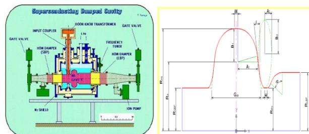
Figure 6: Structure of 500 MHz SRF cavities for IHEP
