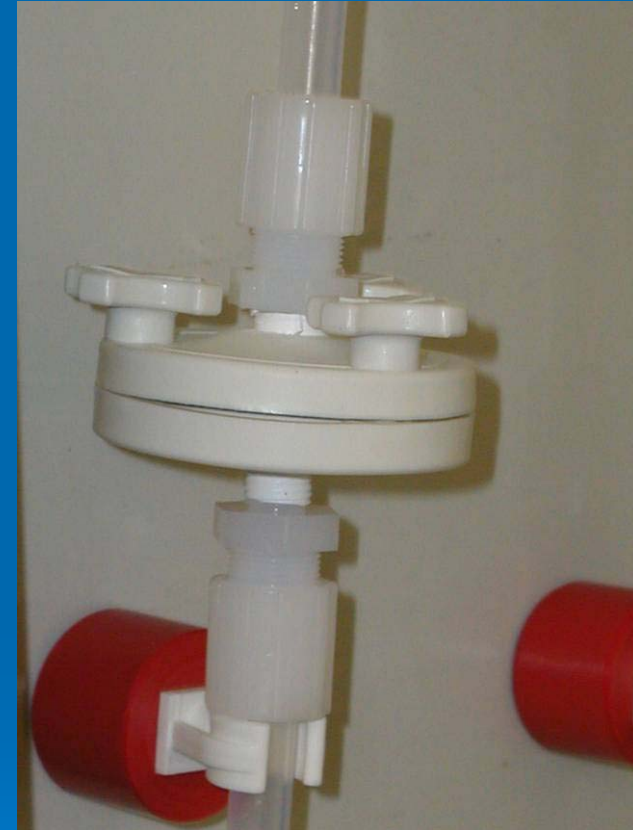
Particle filter \leq 2 \mu\text{m} in HPR draining line
