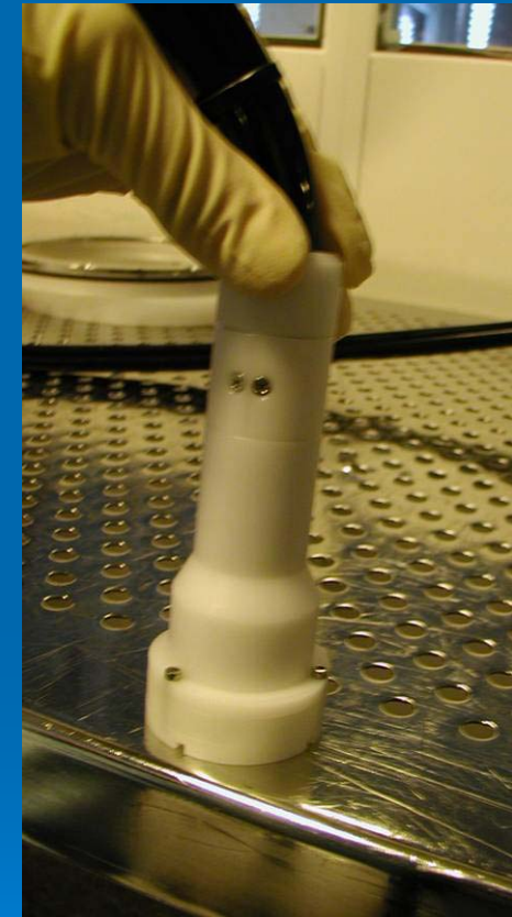
Particle detection on a cleanroom table
