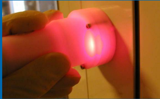
Particle detection on a cleanroom wall
