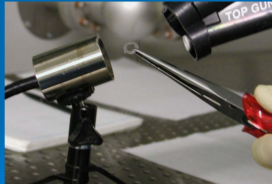
QC of washers before installation to a cavity
