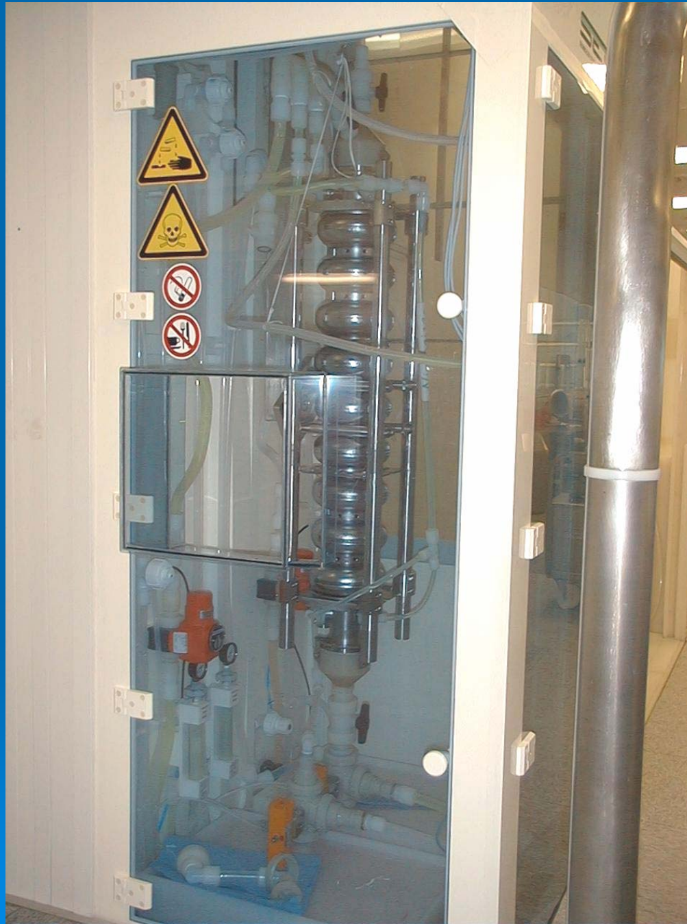
Cavity installed in BCP bench (Buffered chemical polishing
