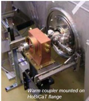
Warm coupler mounted on HoBiCaT flange
