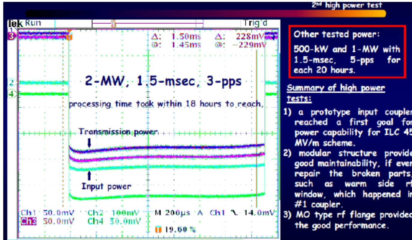
High power test demonstrated that couplers can successfully operate with pulse 1MW x 1.5 x 5pps and 2MW x 1.5ms x 3pps for matching load and pulse 500kW x 1.5ms x 5pps for short. Effect of multipactor is weak. Upper limit of multipactor is about 200 kW.
