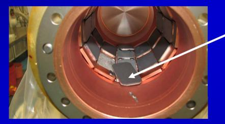
Two ferrite tiles cracked and dropped; found ferrite chips in the cavity beam pipe...
