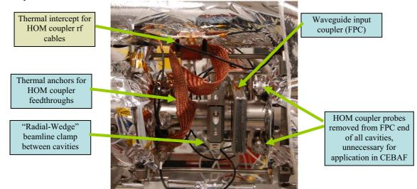
Figure 8. Photograph of HOM coupler region of the cavities with additional thermal anchoring.
