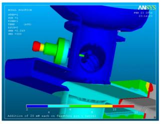
Figure 5. Integrated ANSYS model of Renascence LL cavity endgroup, input waveguide, and HOM coupler feedthrough
