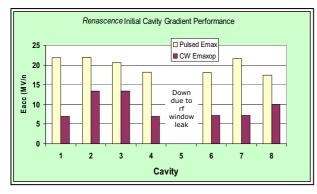
Figure 2. Maximum performance of Renascence cavities on first test.
