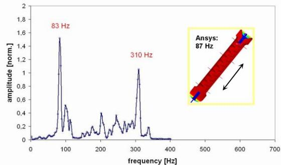
Figure 11: Focus on deep resonances (sweeping method) and corresponding ANSYS simulation, showing the basic longitudinal mode between fixed ends.
