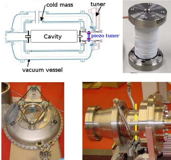
Figure 4: Scheme of the cryostat with tuner positioning on top right, a piezo from Physical Instruments (PI) top left, the mechanical tuner bottom left and beam pipe were piezo tuner shown in fig. 5 will be included close to the cooling loop in the middle (dotted line).
