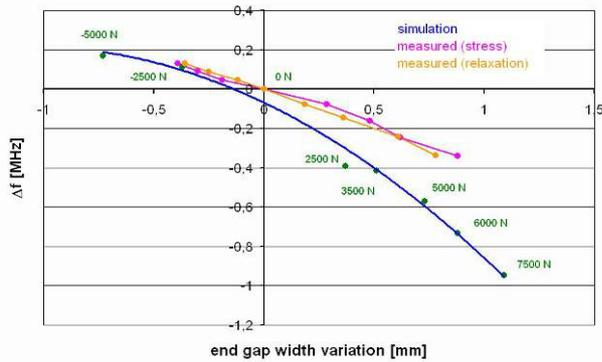
Figure 2: Simulated and measured rf-response.
