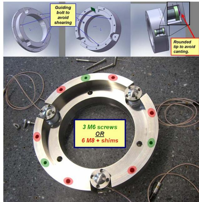
Figure 5: Scheme of the piezo tuner on top and one part of the tuner carrying the three piezo actuators below.
