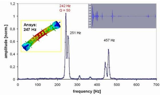
Figure 9: Measured resonances between 200 and 500 Hz. A graphic data output of an ANSYS simulation shows the displacements encoded in colours of the basic transverse mode between fixed ends measured at 242 Hz. The simulated value is 247 Hz. The recorded wave data during sweeping are displayed on top right of the graph.
