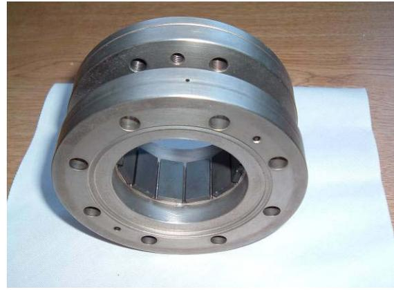
Fig 6. Ferrite HOM absorber at MIT-Bates
