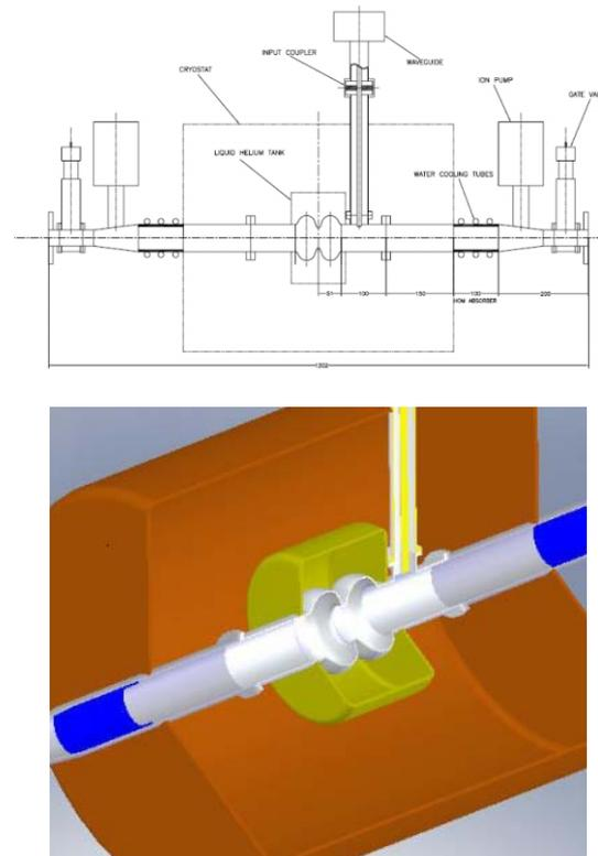
Fig.1. A schematic of the 2.85 GHz SRF cavity with a high RF power input coupler and HOM absorber
