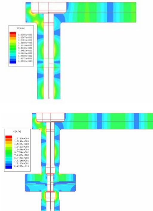
Fig 7. Straight Coaxial RF Coupler Section and Tapered Coaxial Coupler Section.
