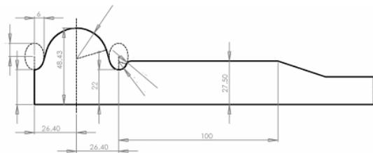
Fig 3: Cavity configuration after several series of optimization
