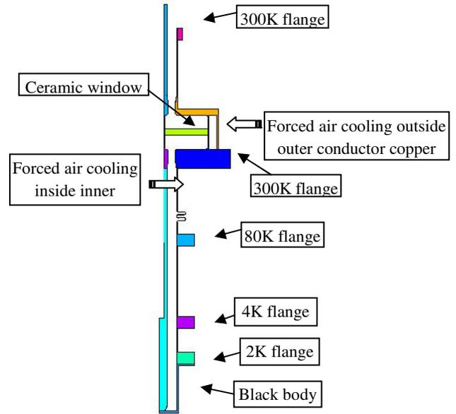
Fig 8. Thermal model for tapered coax coupler
