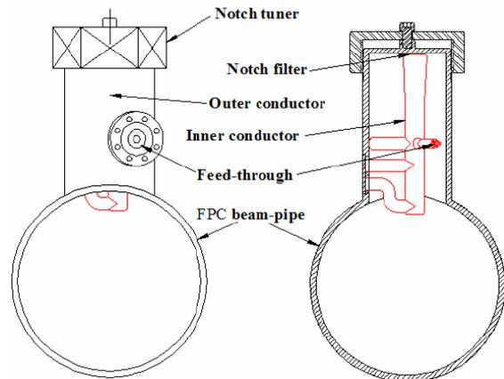
Figure 3: PEPF HOM coupler and cross-section on the FPC beam-pipe.
