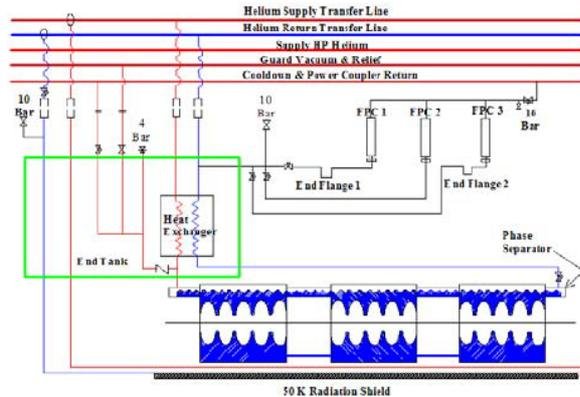
Figure 5: Cryogenic circulation schematic of the PEFP Low beta cryomodule. The blue colour means the supply coolant or cold helium liquid; and the red colour means the return coolant.
