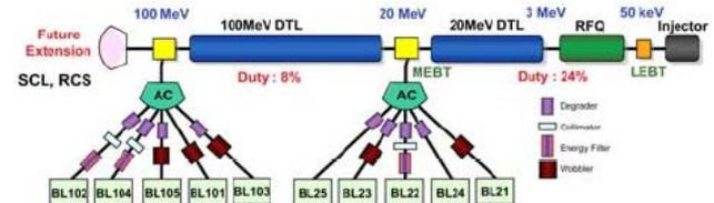
Figure 1: Schematics of the PEFP 100 MeV linac and beam line facilities.
