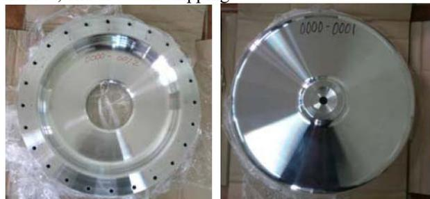
Figure 7: A female die and a male die for the central cells of the PEFP Low-beta cavity.
