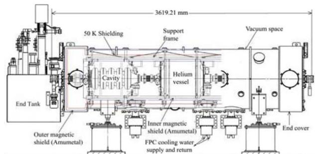
Figure 6: PEFP low beta cryomodule assembly.
