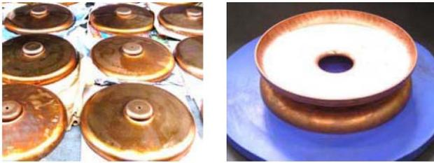
Figure 8: Half cells and a dumbbell of the PEFP prototype copper Low-beta cavity.
