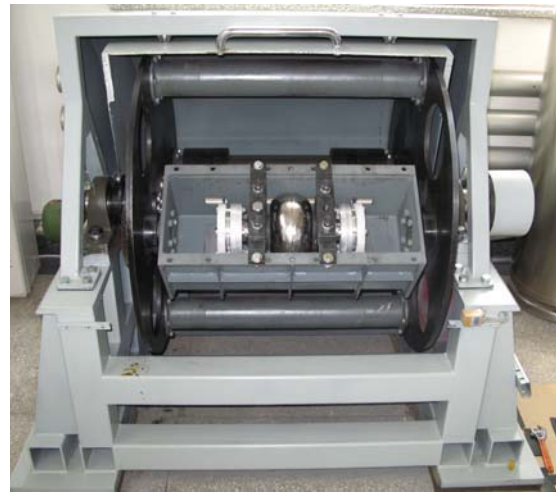
Figure 4: Machine for centrifugal barrel polishing at IHEP.
