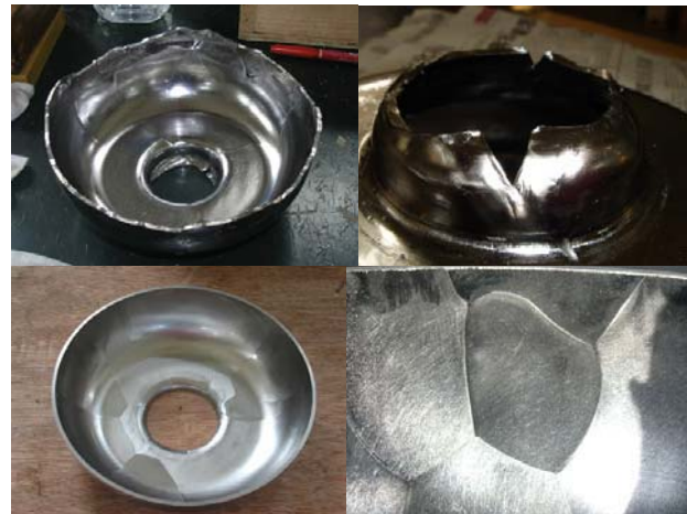
Figure 2: Half-cells after deep-drawing and trimming.
