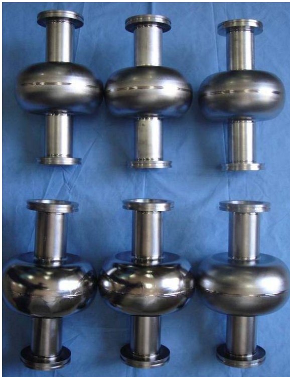
Figure 3: Six low loss cavities welded in Beijing. Three cavities made of fine grain niobium material from Tokyo Denkai. Two cavities made of large grain niobium material from OTIC, Ningxia. Another one made of fine grain material from OTIC, Ningxia and just for electron beam welding test.
