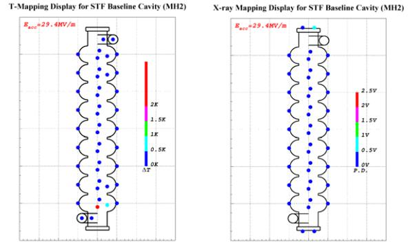
Figure 12: T-mapping and x-ray mapping.
