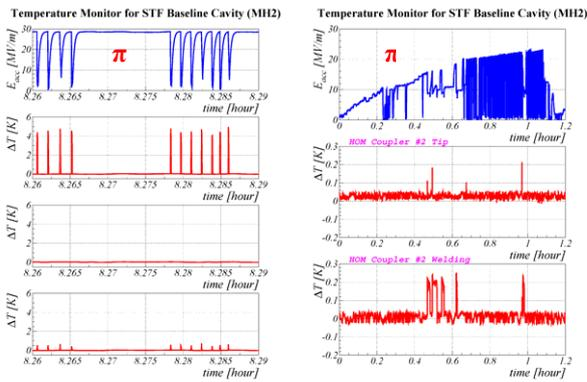
Figure 10: Expanding temperature monitoring around cell and HOM coupler.
