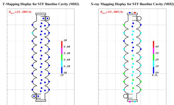
Figure 6: Temperature and x-ray mapping display.
