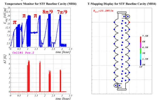
Figure 7: Temperature monitoring and mapping display.
