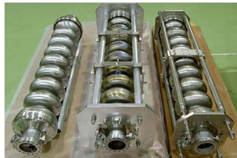
Figure 1: The STF Baseline 9-cell Cavity.
