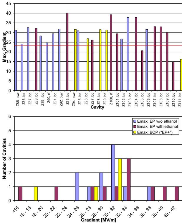
Figure 1: Maximum gradient of 27 cavities (top) and distribution of maximum gradient (bottom) depending on preparation
