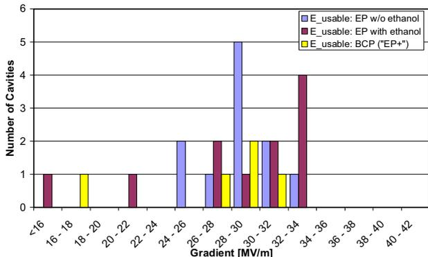
Figure 2: Distribution of usable gradient depending on preparation
