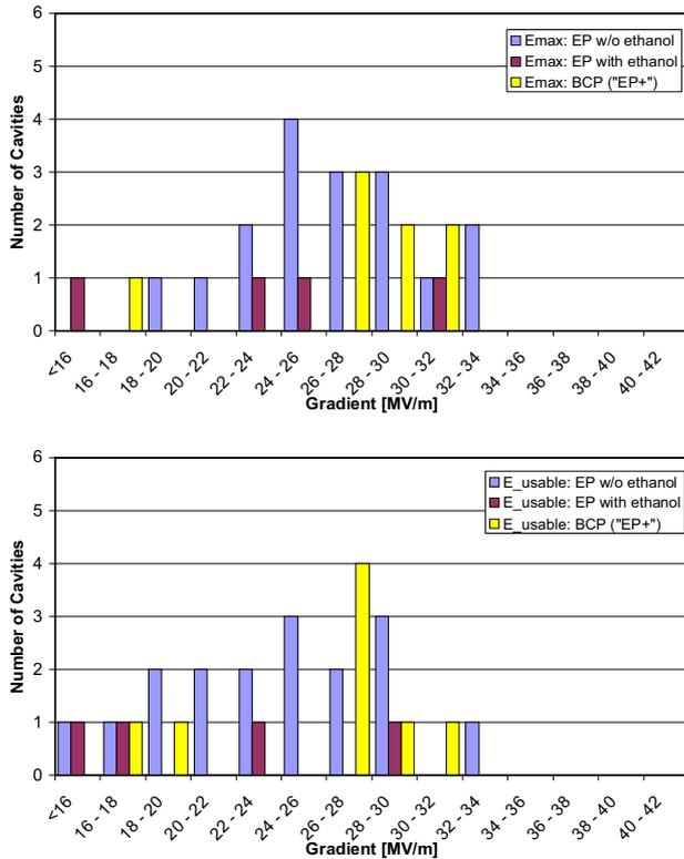
Figure 3 Distribution of maximum (top) and usable (bottom) gradient after first preparation
