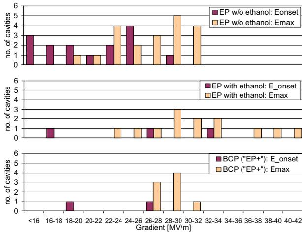
Figure 5: Comparison of  $E_{acc,max}$  and  $E_{acc,onset}$  for EP without ethanol rinse (top), EP with ethanol rinse (middle) and final short BCP treatment (cavities Z110 + Z111 not included)
