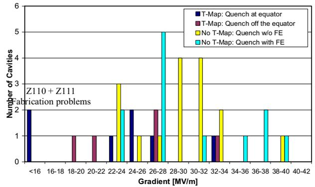
Figure 4: Analysis of quench gradients
