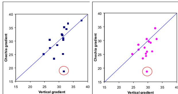
Figure 6: Comparison of horizontal and previous vertical test result for both maximum and usable gradient
