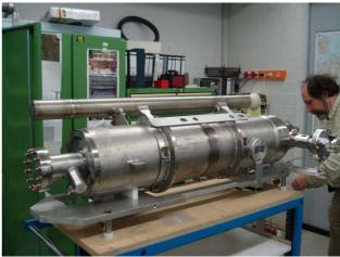
Fig. 6 - Cavity integrated in the modified helium tank in Halle III machine shop at DESY
