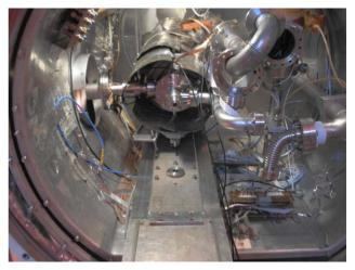
Fig 10 – The Z86 cavity inside CHECHIA.
