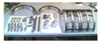
Fig. 7 – Tuner components before assembling
