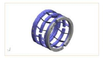
Fig. 4 - The additional adaptation rings, in grey, installed for the Slim tuner
