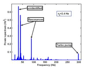
Figure 10: Power spectrum of microphonics
