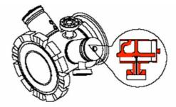
Figure 8: HOM feedthrough of the TESLA cavity. There is a SMA connector with a tip coupling capacitive to the F-part of the HOM antenna of the cavity.
