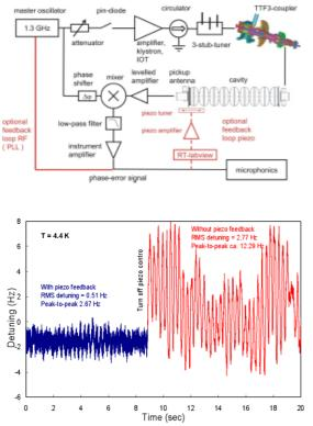
Figure 11: Electrical setup (upper figure) of the microphonics measurement and feedback loop. Lower figure shows the Microphonic detuning (red) versus time and the reduction (blue) by closing the feedback loop.
