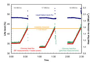
Figure 3: By using a electrical heater the total losses (red) of the heater and the dissipated cavity wall losses for different field settings (blue) were increased. The quenching occurred at total power of 35 W or 1.53 W/cm<sup>2</sup> in the chimney.
