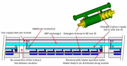
Figure 5: Design of a CW cryo module
