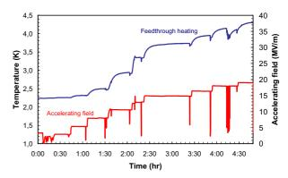
Figure 9: Temperature rise of the sapphire HOM feedthroughs and accelerating field versus time of the S33 cavity in CW operation. The HOM heating is at a moderate level.
