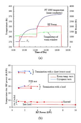
Figure 7: CW measurements at the TTF-III type coupler. (a) Example of PT1000's temperature versus time. Measurements were made with HoBiCaT cold and the waveguide shortened. (b) Summary of all tests.
