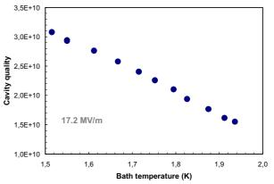
Figure 6: Unloaded quality factor of the TESLA cavity versus bath temperature. At low temperatures the quality factor increases. There is no saturation by other loss mechanisms seen at these measurements at HoBiCaT.
