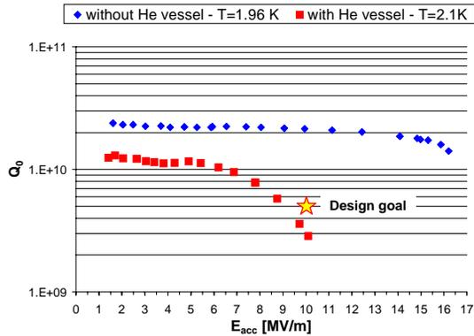
Figure 2: SNS  $\beta = 0.61$  vertical test results.
