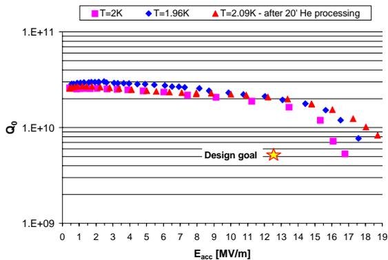
Figure 3: SNS  $\beta = 0.81$  vertical test results.
