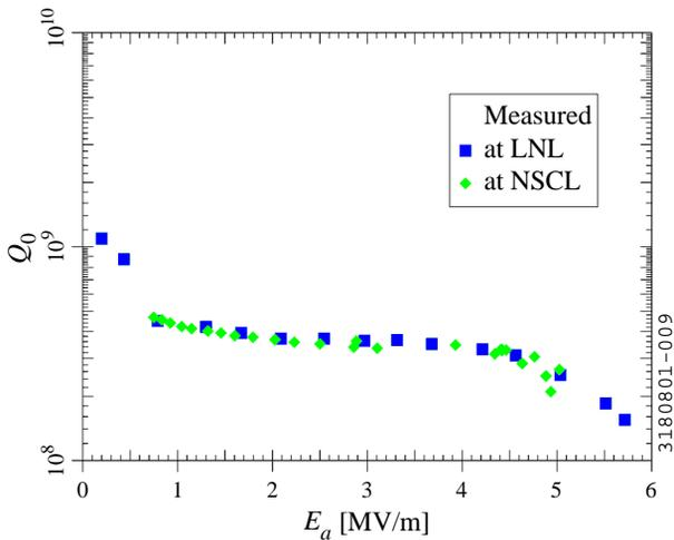
Figure 10. Measured dependence of  $Q$  on accelerating gradient for 80 MHz cavity, before and after etching at NSCL.
