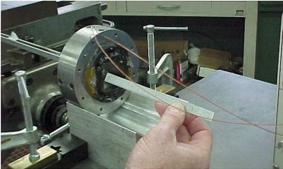
Figure 11. Superconducting quadrupole during magnetic field mapping at room temperature.
