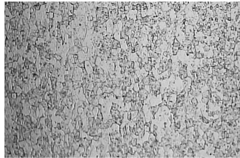
Figure 13. Grain structure of RRR Nb.
