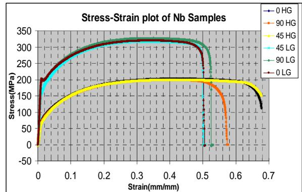
Figure 12. Stress-strain plot of Nb.
