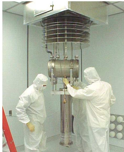
Figure 9. QWR installed on insert.
