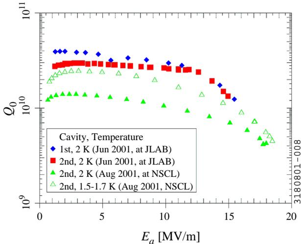
Figure 6. Measured dependence of  $Q$  on accelerating gradient for the RIA cavity.
