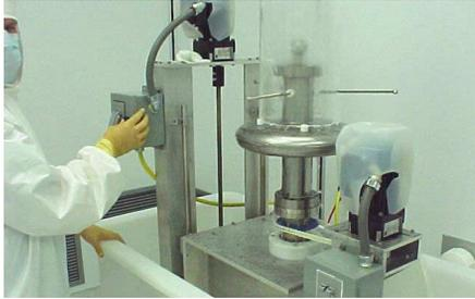
Figure 5. High pressure rinsing of RIA cavity.
