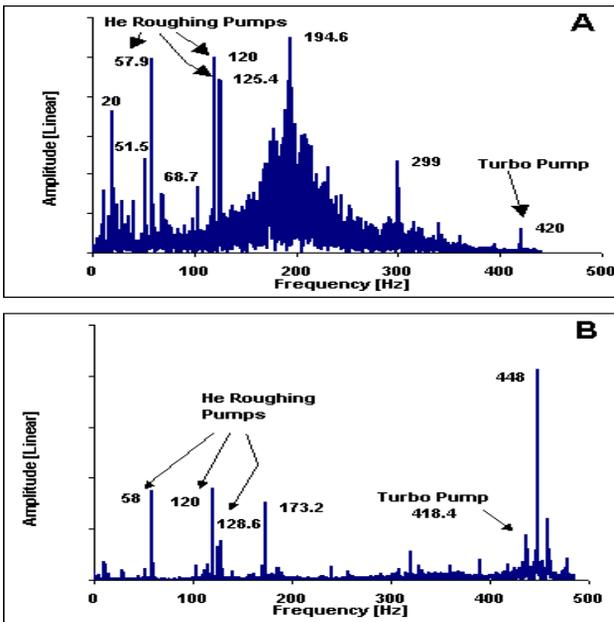
Figure 7. Microphonics spectrum from FFT of (A) cavity's phase lock loop/error signal, and (B) accelerometer on top of Dewar.
