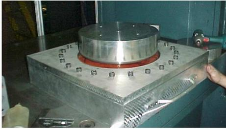
Figure 4. Dies for deep drawing of RIA half-cell.
