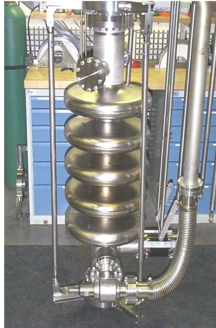
Figure 1: APT 5-cell cavity set on the cryostat insert. Details of the tests are described in [2-4].
