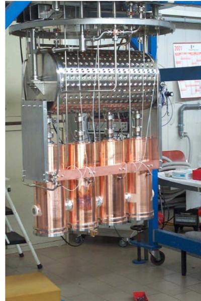
Fig. 1 : 160 MHz, medium  $\beta$  cryostat equipped with four Nb/Cu sputtered resonators
