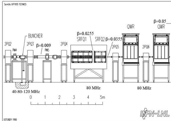
Figure 2: The PIAVE linac layout.
