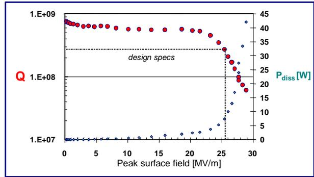
Fig. 4: SRFQ2 rf test results.
