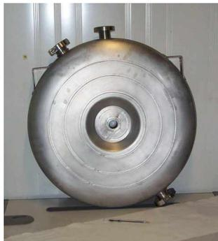
Fig. 7: The TRASCO 352 MHz reentrant cavity prototype.
