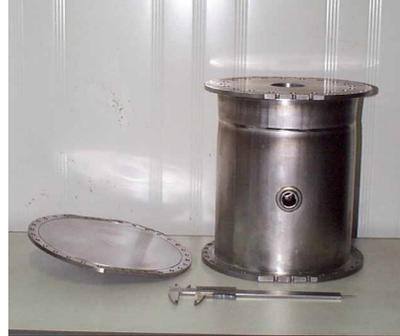
Fig. 8: The 352 MHz quarter wave cavity.
