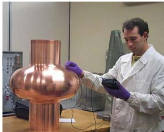
Figure 4: INFN 500 MHz cavity by spinning from tube.
