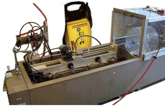
Figure 10: A new automated high-pressure rinsing system for the surface preparation of superconducting cavities.
