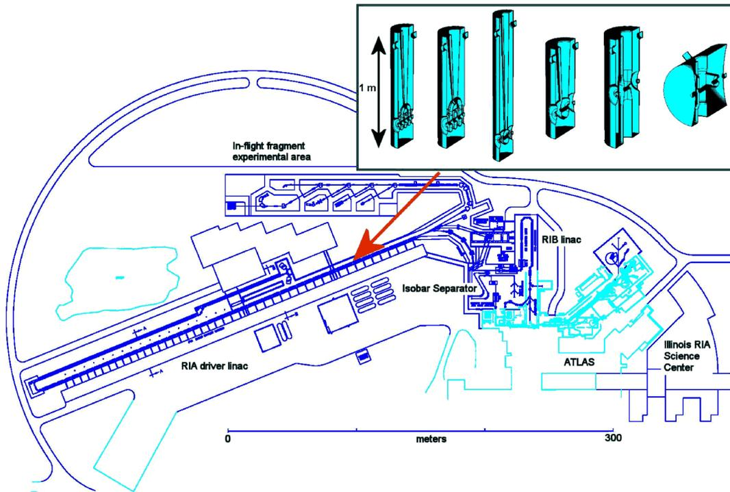
Figure 5: Layout for the Rare Isotope Accelerator at Argonne National Laboratory. The inset shows a set of niobium drift-tube cavities suitable for  $0.02 < \beta < 0.6$  for the RIA driver linac.
