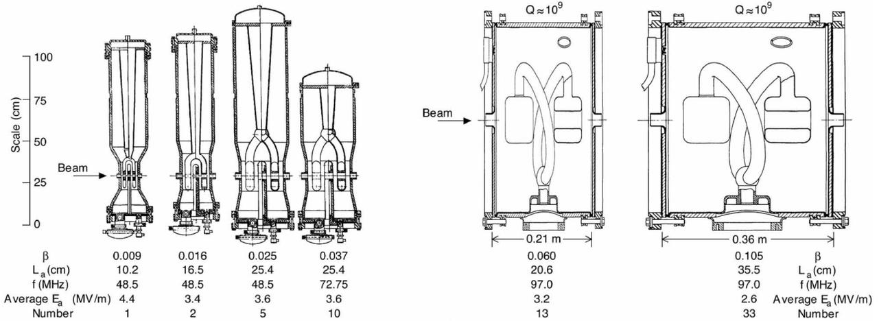
Figure 3: Cutaway view of the quarter wave resonators used in the Positive Ion Injector (left) and the split-ring resonators used in the ‘booster’ and ‘ATLAS’ sections of the accelerator.
