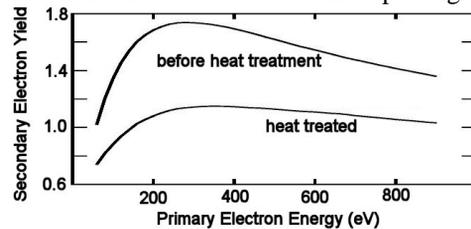
Figure 12: Secondary electron yields from a niobium sample before and after annealing at 250 °C for 19 hours.
