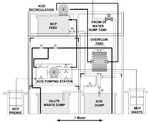
Figure 11: A new facility for buffered chemical polish (BCP) of superconducting rf cavities.
