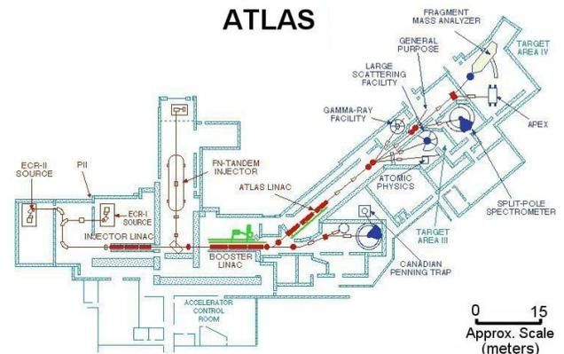
Figure 2: Top view of the ATLAS facility containing three major sections of superconducting LINAC.
