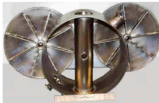
Figure 7: A 350 MHz  $\beta=0.4$  prototype spoke cavity prior to welding on the end plates.
