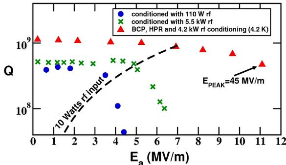
Figure 8: Top – Spoke cavity performance following BCP, high-pressure rinsing and rf conditioning compared to earlier results with only rf conditioning (bottom). The peak surface electric field,  $E_{PEAK} = 45$  MV/m.
