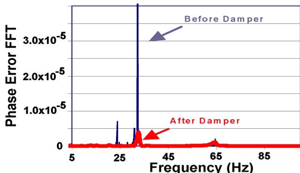
Figure 4: Phase error for a  $\beta=0.016$  resonator before and after installation of a vibration damper.
