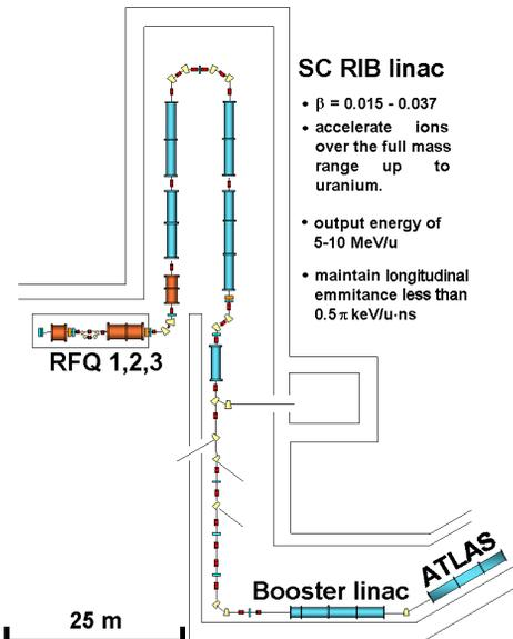
Figure 6: Design for a post accelerator for the Rare Isotope Facility based largely on superconducting rf quarter-wave cavities.
