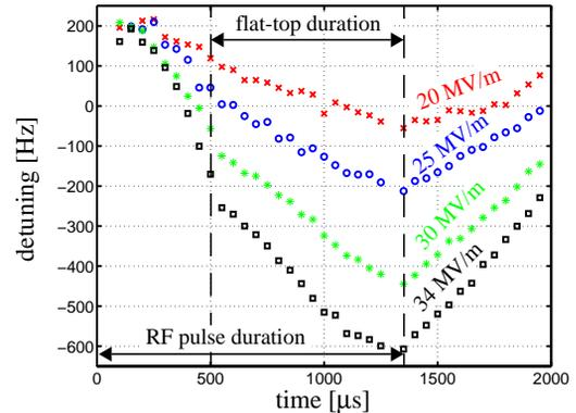
Fig. 1: Typical Lorentz force detuning during pulsed operation of a TTF 9-cell cavity at different flat-top gradients.
