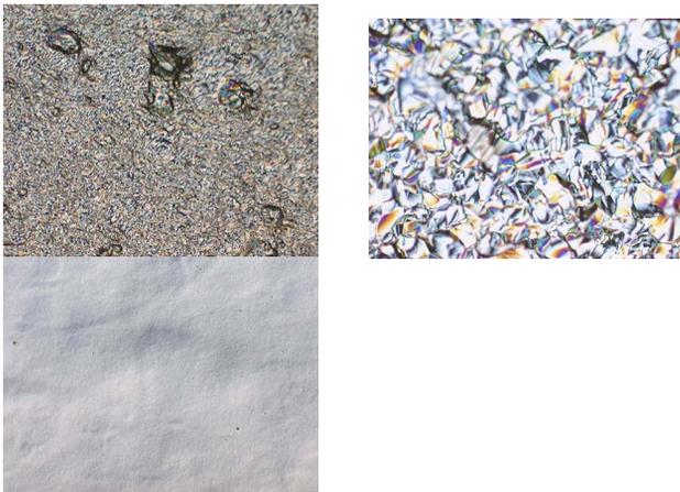
Pic.3: Pictures in order raw sheet material, after 120μm BCP, after 120μm EP [Ref.7]
