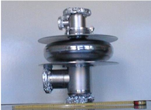
Figure 3 700 MHz mono cell w. SS helium tank end caps
