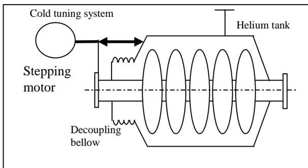
Figure 1 Principle layout of the cavity cold tuning
