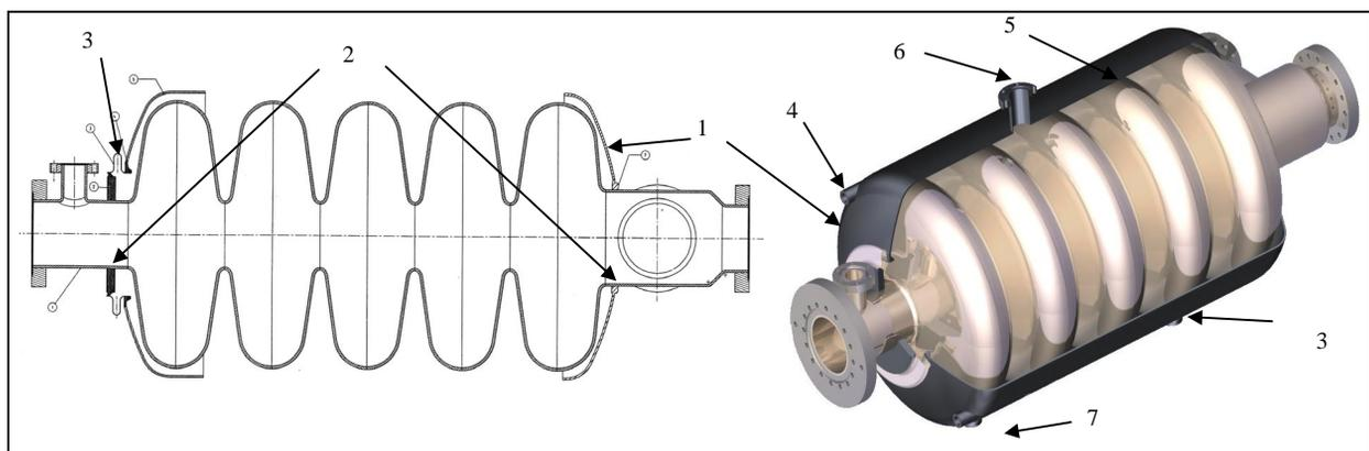
Figure 5 Helium tank design
