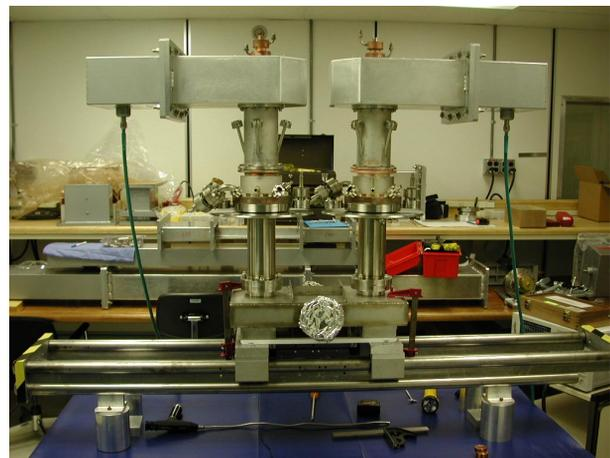
Figure 6: FPCs mounted on connecting waveguide
