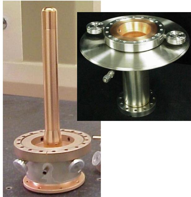
Figure 2: Window and inner conductor (a) and outer conductor (b)
