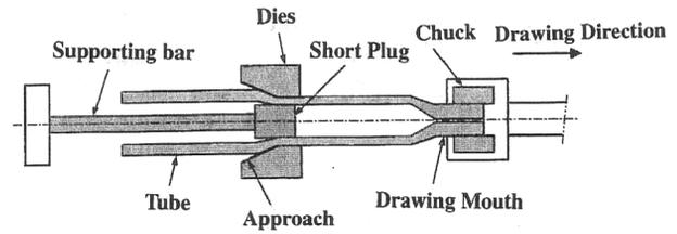
Figure 10: Principle of tube drawing technology
