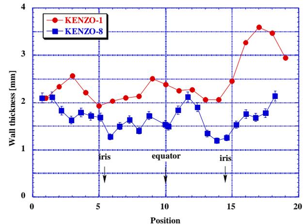
Figure 2: Wall thickness distribution of Nb/Cu spun cavities
