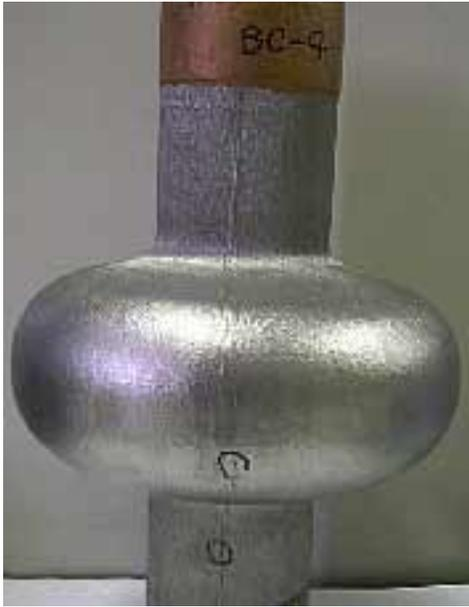
Figure 8: Cracks on beam welding seam in BC-4 cavity
