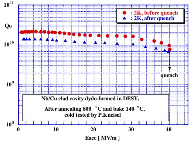
Figure 5: Excellent high gradient performance of Nb/Cu clad cavity.
