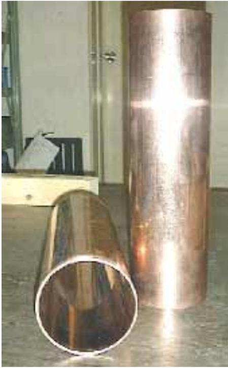
Figure 12: Completed Cu/Nb/Cu sandwiched tubes by drawing technology
