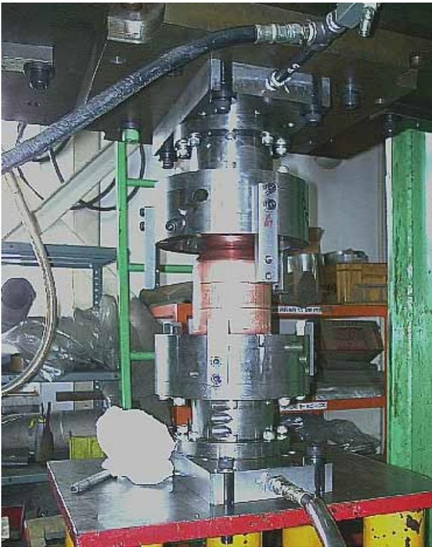
Figure 14: Hydro-forming of a copper tube
