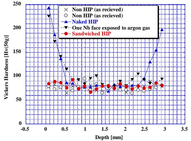
Figure13: Hardness (Vickers) in cross-section of materials after HIP process
