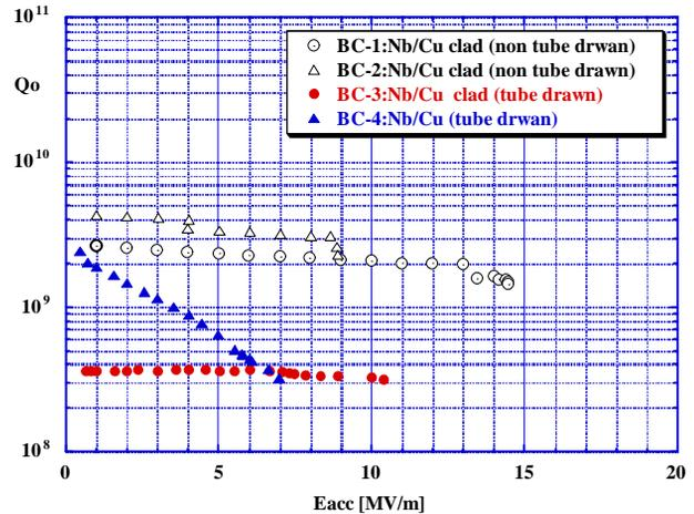
Figure 7: Excitation curves with Nb/Cu clad cavities hydro-formed in Toshiba
