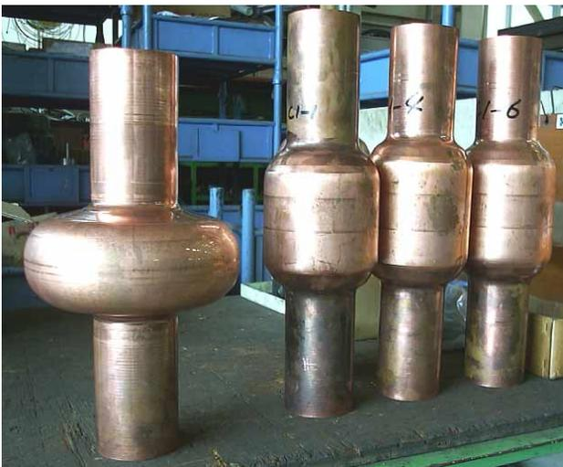
Figure 15: Successfully hydro-formed Cu cavity (left) and swaged tubes for hydro-forming (right)
