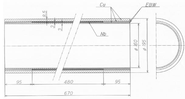
Figure 9: Primary clad tube design for HIP
