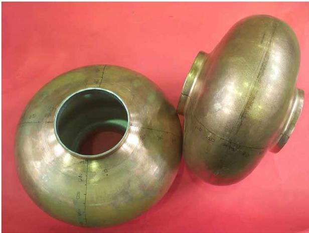
Figure 3: 1300MHz Nb/Cu clad cavity cells fabricated at DESY by hydro-forming
