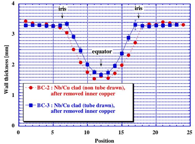
Figure 6: Distribution Wall thickness in hydro-formed Nb/Cu clad cavities
