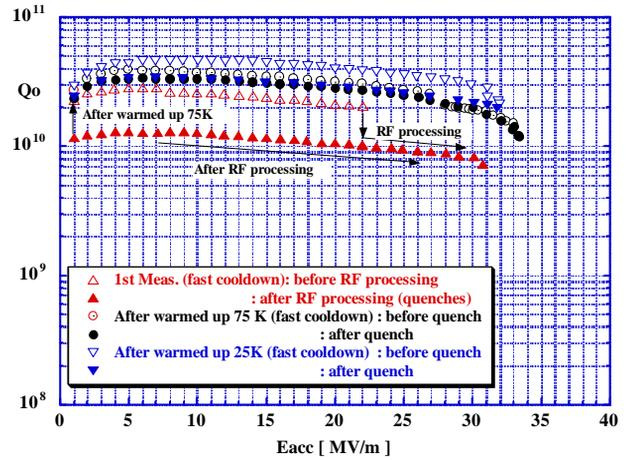
Figure 4: First result in KEK of a Nb/Cu clad cavity fabricated by hydro-forming at DESY
