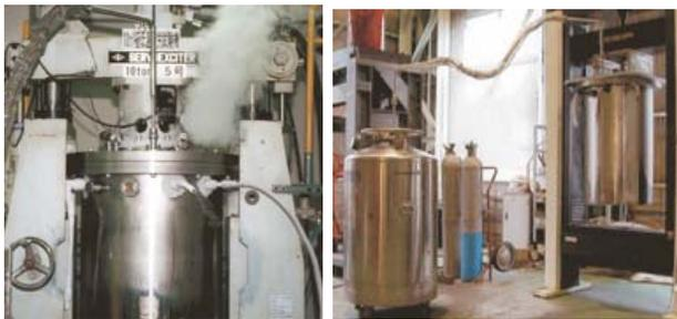
Fatigue pre-crack at 77 K    Fracture toughness test at 4 K
