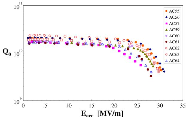
Figure 1: Performance of TESLA cavities delivered by ACCEL
