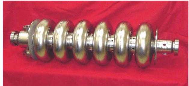
Figure 2: Prototype of medium beta cavity for SNS produced by JLAB (courtesy Jefferson Laboratory)
