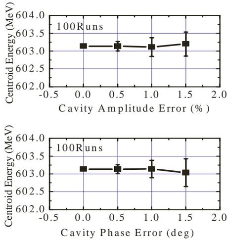
Fig.7 Energy jitter of the beams obtained from the rf control error analysis
