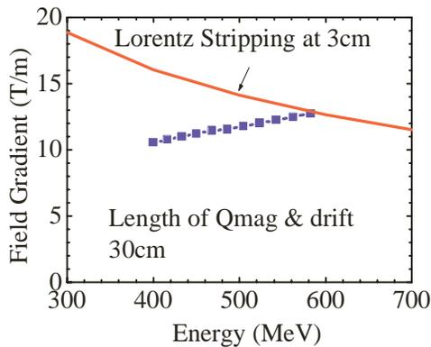
Fig.3 Field gradient of the Q magnet and the Lorentz stripping limit
