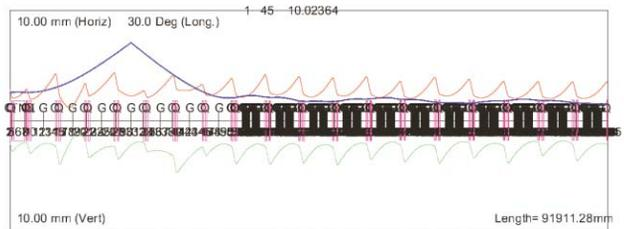
Fig. 9 Results of the MEBT study. Beam envelopes from the last ACS section to the whole SC linac.
