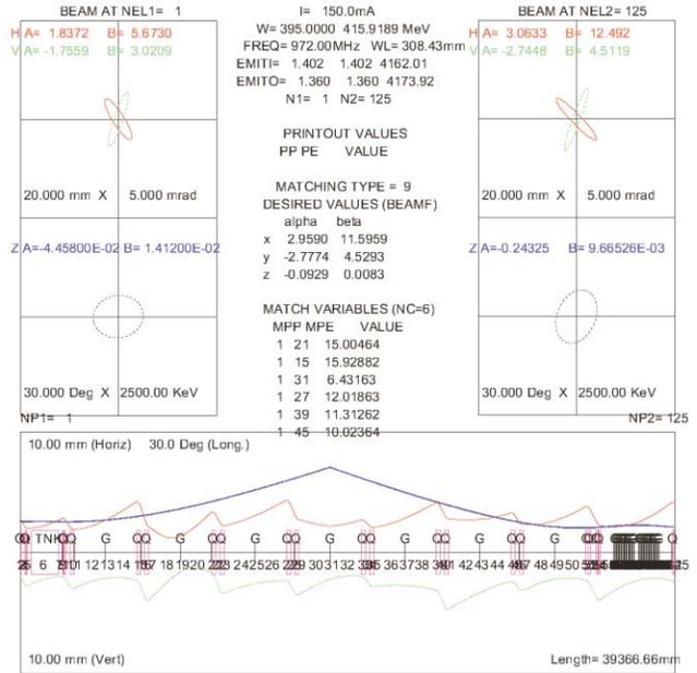
Fig. 8 Results of the MEBT study with TRACE-3D. Phase space plots and beam envelopes from the last ACS section (left) to the 1-st SC section (right).
