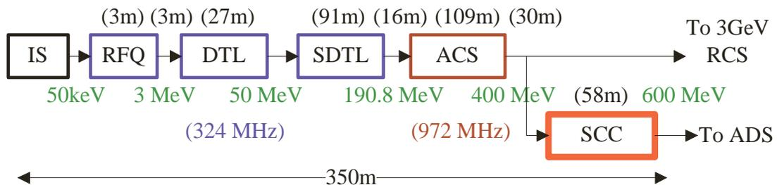
Fig.1 Block diagram of the linac
