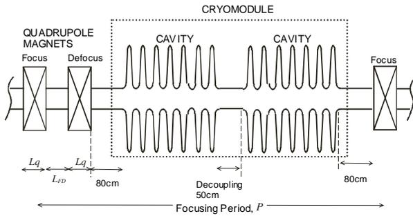
Fig.2 Lattice structure of the SC linac
