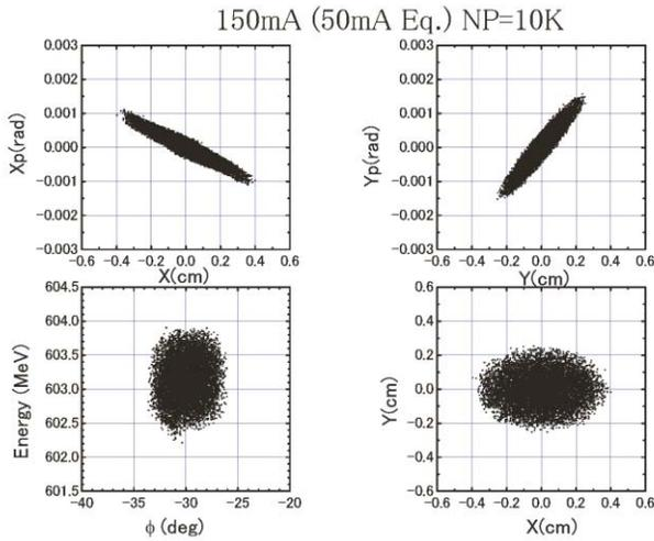
Fig.6  $x-x'$ ,  $y-y'$ ,  $W$ - $\phi$  phase space plots and  $x$ - $y$  spatial plots at the exit of the SC linac
