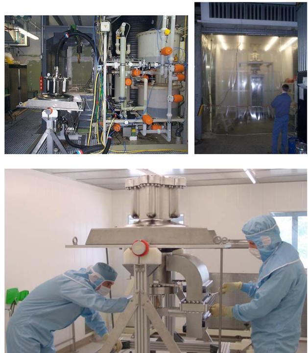
Figure 4: Preparation at ACCEL of a 500 MHz cavity for a vertical test. up left: closed loop BCP, up right: high pressure rinsing, below: clean room assembly.
