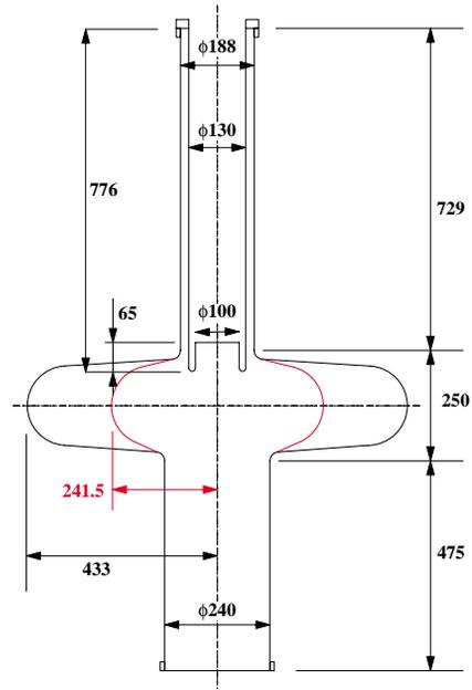
Figure 2: Simplified inner conductor attached to the cavity. Red line represents the cavity cell of short axis.
