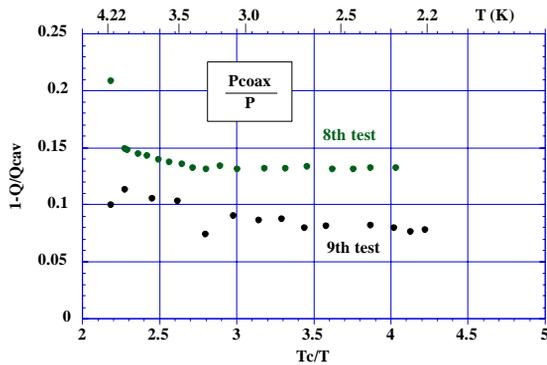
Figure 13: Conductor loss ratio.
