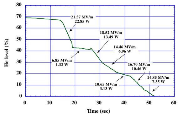
Figure 7: Liquid helium level and conductor losses at several fields.
