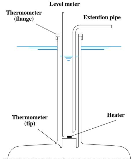
Figure 6: Setup for calorimetric measurement.
