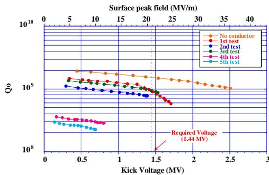
Figure 4: Cold test results.
