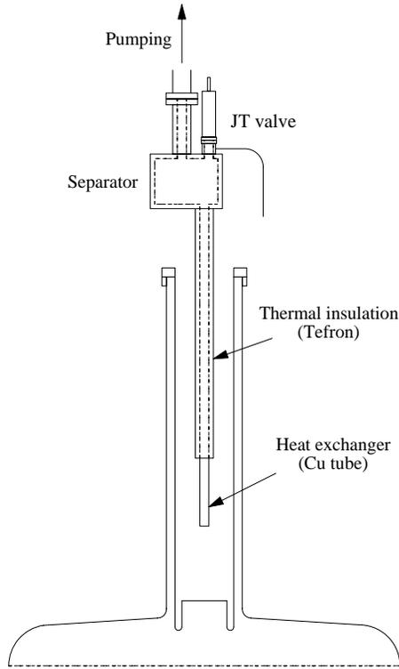
Figure 12: Sub-cooler set in the conductor.
