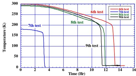
Figure 10: Cool-down curves from 6th to 9th cold tests.
