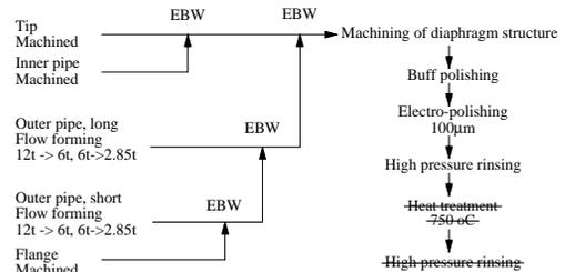
Figure 3: Fabrication flow and surface treatments of the simplified inner conductor.
