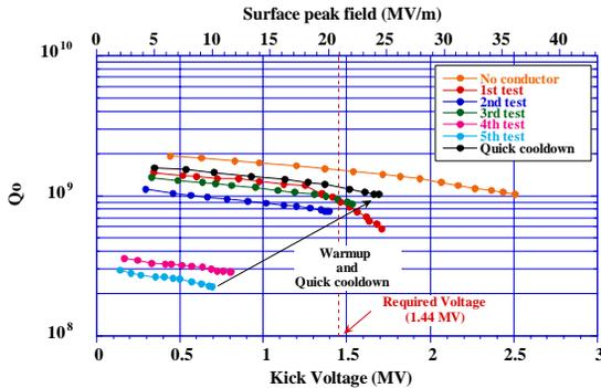
Figure 9: Recovery from Q-degradation.
