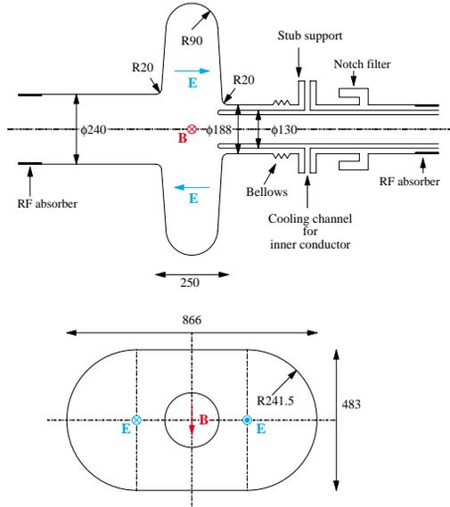
Figure 1: Squashed cell and co-axial beam pipe coupler.
