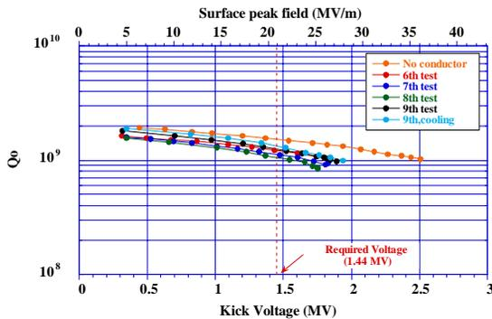
Figure 11: Cold test results from 6th to 9th tests.
