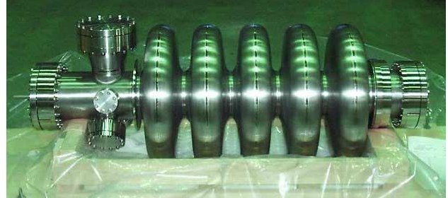
Fig. 1 600MHz 5-cell cavity ( \beta=0.604 )
