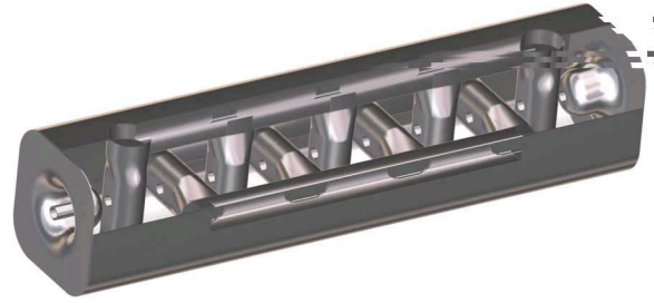
Figure 5: 10-Gap SCH with Bars (320 MHz, \beta=0.3 )
