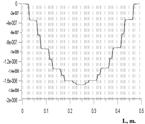
Fig. 9 Deformation of accelerating cavity with the fixed bottom and top flange at the thickness of a wall of 2 mm.
