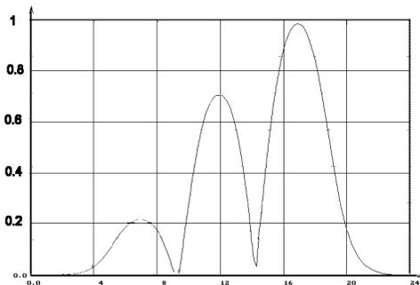
Fig.3. Distribution of EM field along the axes of grouping cavity
