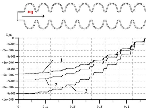
Fig. 8 Deformation of accelerating cavity with the fixed bottom flange at various values of thickness of a wall
