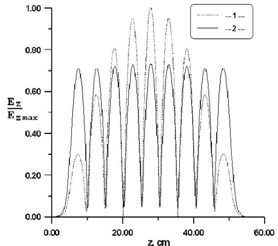
Fig.4. Distribution of EM field along the axes of accelerating cavities: 1-before tuning; 2- after tuning
