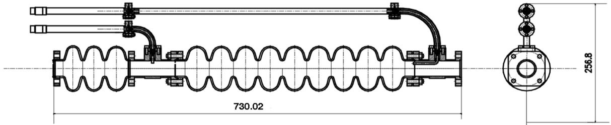
Fig.2. RF superconducting structure for SVAAP
