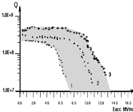
Fig.11. Dependence for  $Q = f(E_{acc})$  of the SVAAP-shape cavity (1,3) for 3 GHz, 2-for 2.45 GHz and TJNAF-shape cavity (5) for 1.3 GHz.
