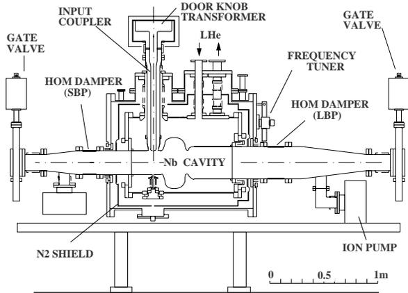
Figure 1: A cross sectional view of the 508 MHz SC module for KEKB.
