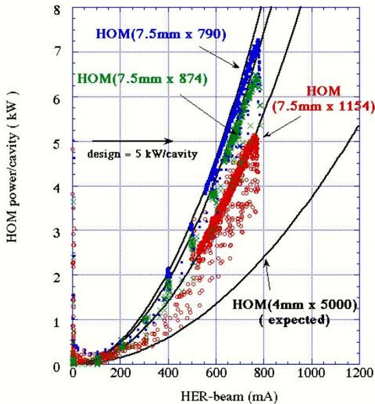
Figure 7: The total power absorbed by the ferrite dampers of D11-cavities. Solid lines show the calculated power for the bunch length of 7.5 mm.
