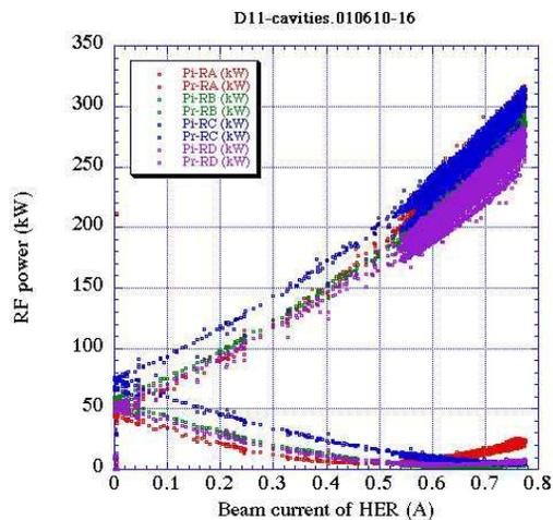
Figure 6: RF input and output power of D11 cavities as the beam intensity.
