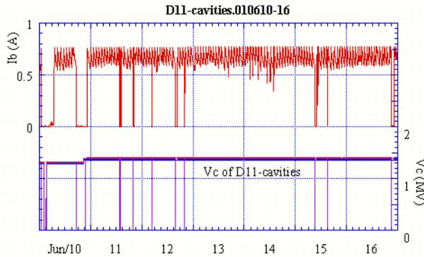
Figure 3: An example of one-week-operation of KEKB and an accelerating voltage of SC cavities.
