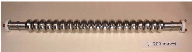
Figure 2: Photograph of a 20-cell cavity.
