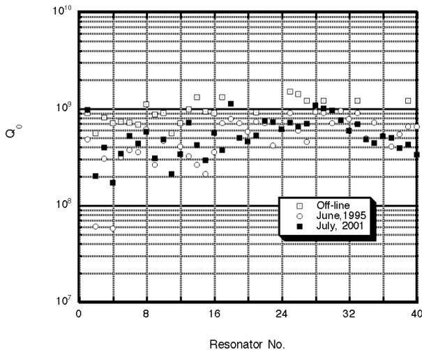
Fig. 3 Q factors at 1 MV/m measured in off-line test, in June 1995 and in July 2001
