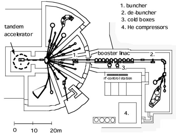
Fig.1 Layout of the JAERI Tandem and its booster
