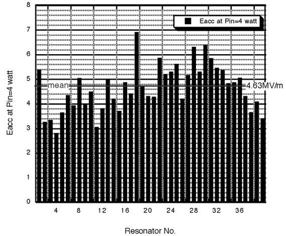
Fig. 4 Field gradients  $E_{acc}$  at the rf input of 4 watts measured in July 2001
