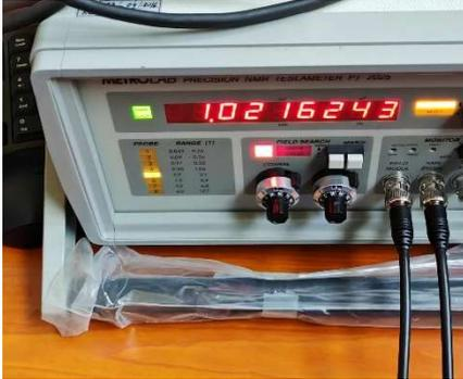
Figure 1: Field intensity measured by NMR probe.
