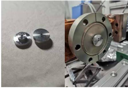
Figure 5: Eccentric disc and fitting between disc and coupler hole.
