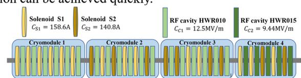
Figure 2: Cryomodule composition diagram.
