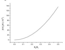
Figure 1: The relative variation of the undulator parameter due to high-order magnetic field. The horizontal coordinate is the ratio of  $B_3$  to  $B_1$ .
