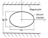
Figure 1: Metallic vacuum chamber and ferromagnetic boundaries.
