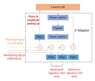
Figure 1: Schematic diagram of the X-Adapter.
