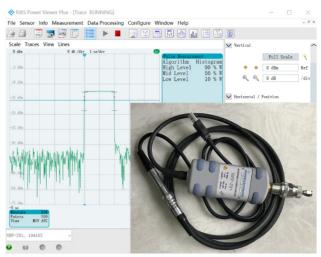
Figure 4: ROHDE&SCHWARZ power meter and its GUI on computer.
