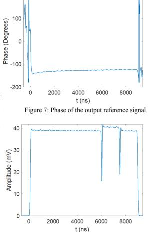
Figure 8: Amplitude of the modulated signal.
