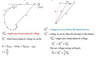
Figure 3: The build up of beam induced voltage in cavity.
