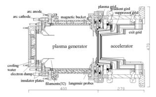
Figure 1: Schematic of high current ion source.
