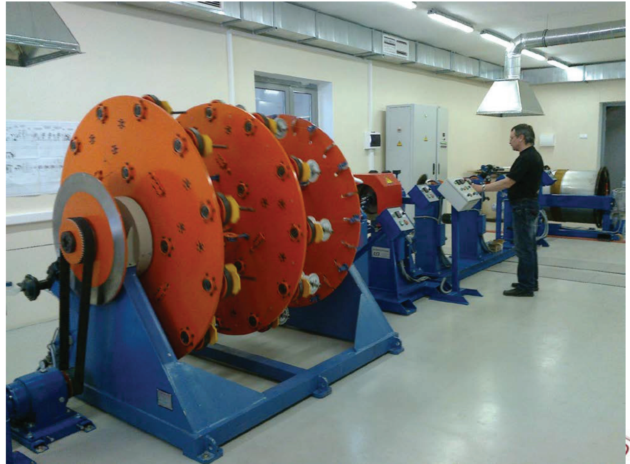
Machine for production SC cable
