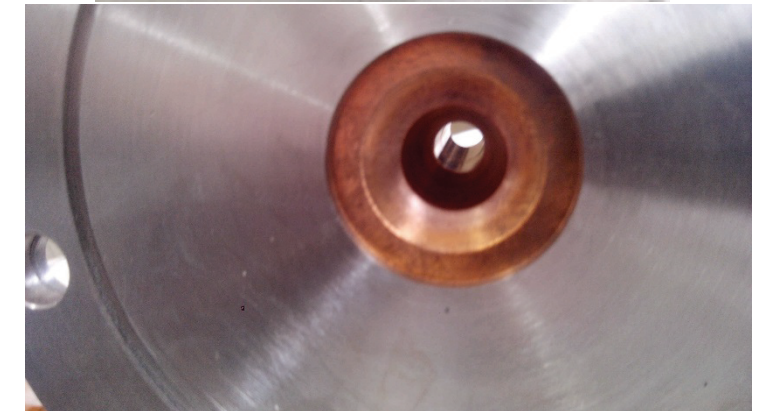
Water cooled diaphragm with 16 mm bore diameter and 120 mm length
