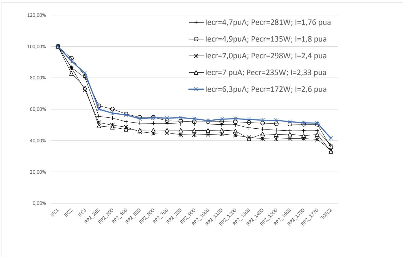
The beam of  $^{52}\text{Cr}^{+10}$  from ECR source with intensity is about 6,3 p $\mu\text{A}$  and accelerated with intensity 2,6 p $\mu\text{A}$ . We can see, that efficiency of acceleration worsen then we increase power input to ECR source.
