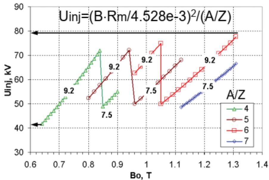
To ensure optimal injection conditions for all range of accelerated ions, two versions of the inflector type A and type B with two magnetic radii of 7.5 and 9.2 cm are used.
