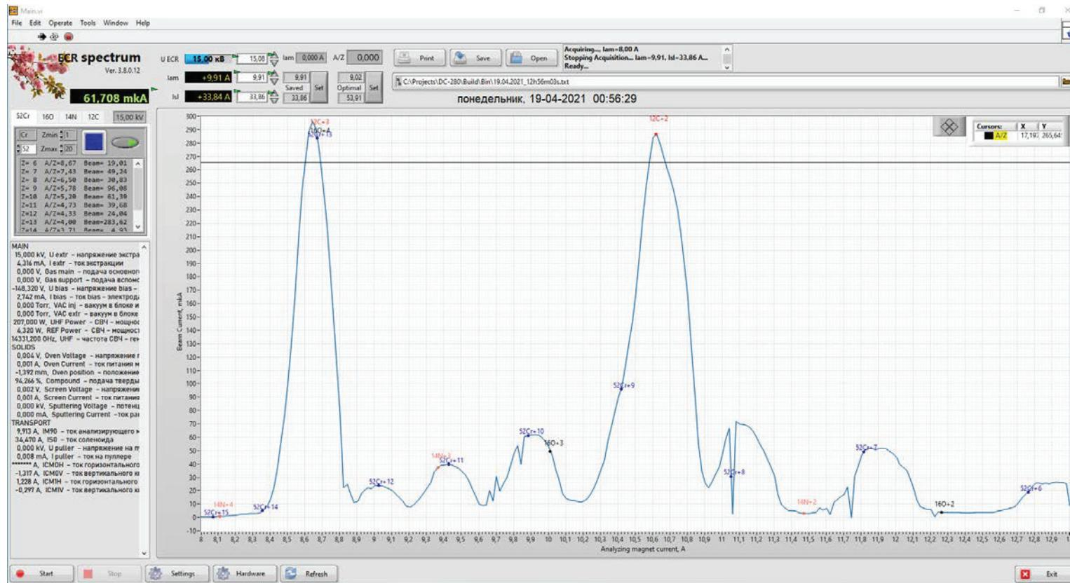
The ions of  $^{52}\text{Cr}$  with a charge of +7, +8, +10 do not contain impurities, but we cannot accelerate ions with a charge of +7 and +8 to the energy required for the experiment.
