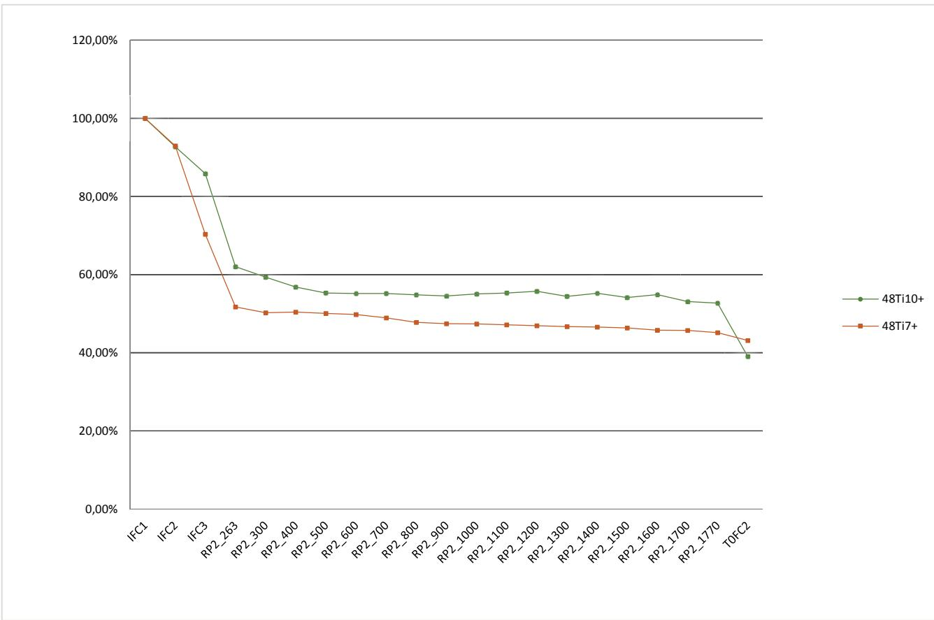
The beam of  $^{48}\text{Ti}^{+10}$  from ECR source with intensity is about 2.5 p $\mu\text{A}$  and  $^{48}\text{Ti}^{+7}$  with intensity is about 3.14 p $\mu\text{A}$  were obtained and accelerated with intensity 1,0 p $\mu\text{A}$  and 0,93 p $\mu\text{A}$  respectively. The total efficiency of transporting the ion beam of  $^{48}\text{Ti}^{10+,7+}$  from the vertical part of the injection to the transport channel is about 40-45%.
