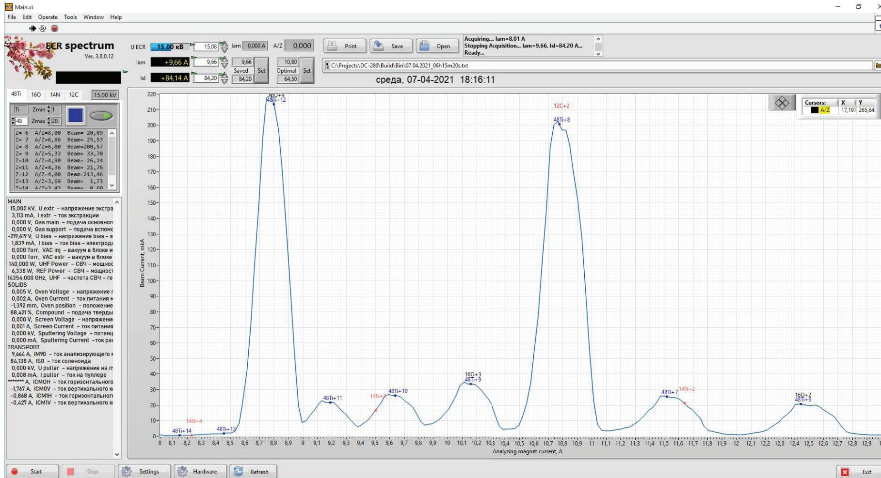
The ions of  $^{48}\text{Ti}$  with a charge of +7, +10 do not have impurities and we can use them in experiments on the synthesis of SHE.
