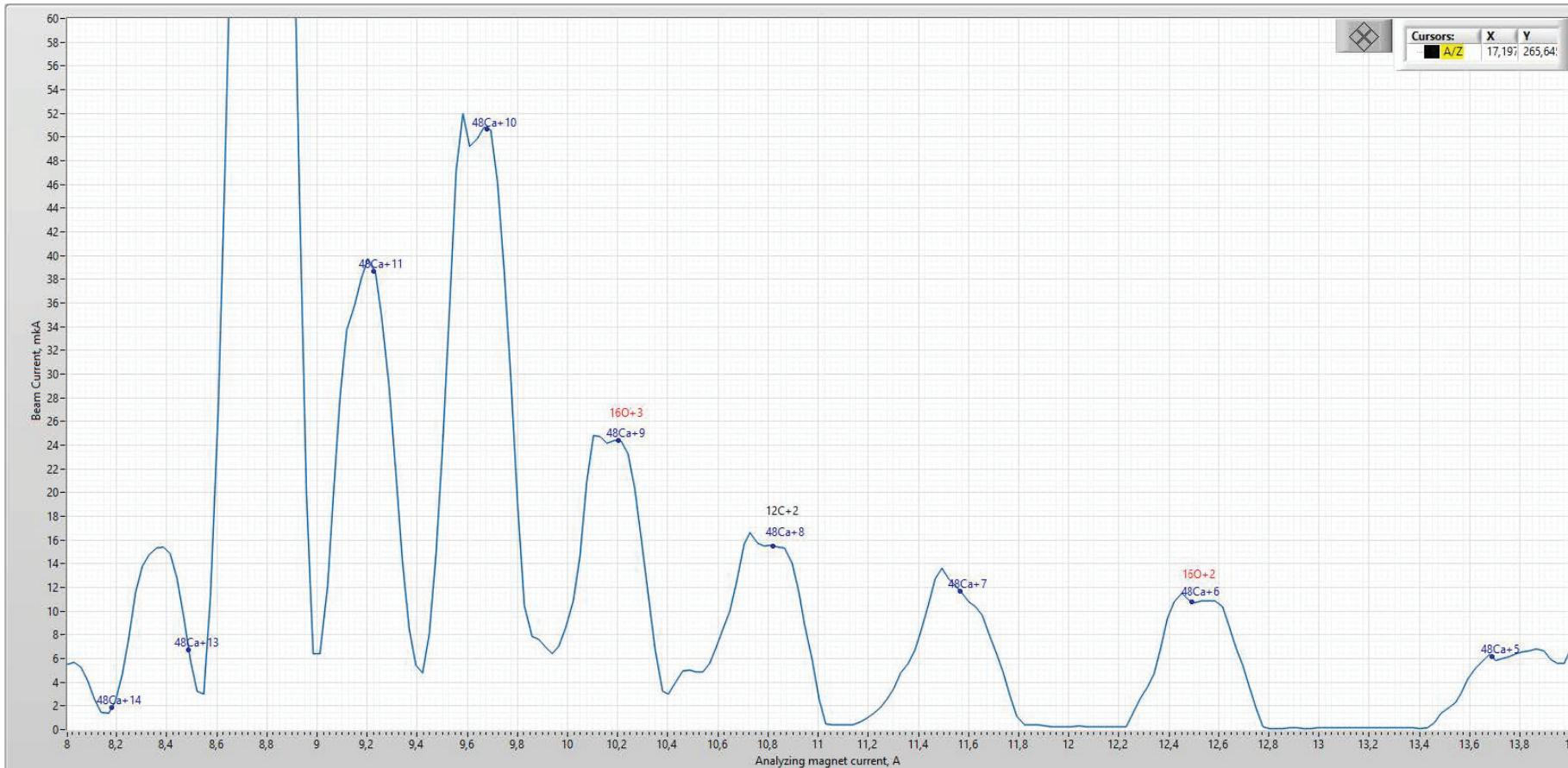
How we can see from the spectrum obtained from the ECR source, ions with charge +7, +10 don't have impurities. Due to the lower consumption,  $^{48}\text{Ca}^{+10}$  was chosen for experiments on the synthesis of superheavy elements.
