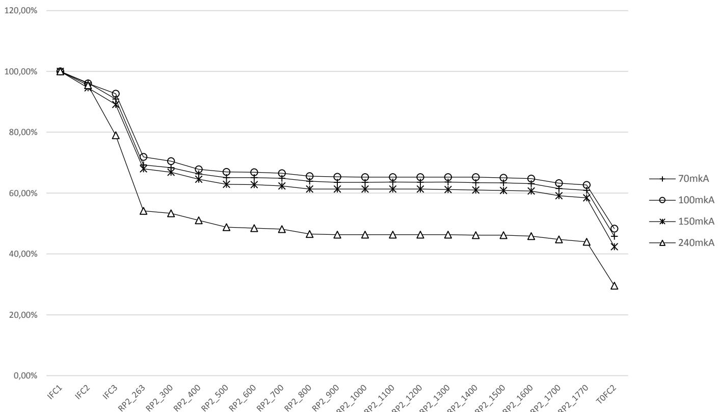
The total efficiency of transporting the ion beam of  $^{48}\text{Ca}^{10+}$  from the vertical part of the injection to the transport channel is about 50%.
