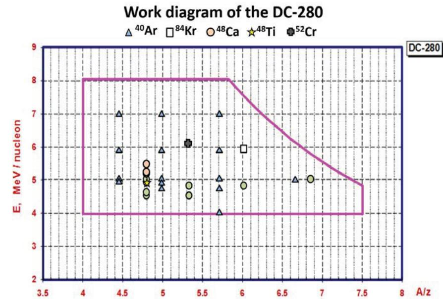
The work diagram of DC-280 cyclotron with marks of tested regimes is presented on Fig.2. The cyclotron has shown reliable and highly effective work.
