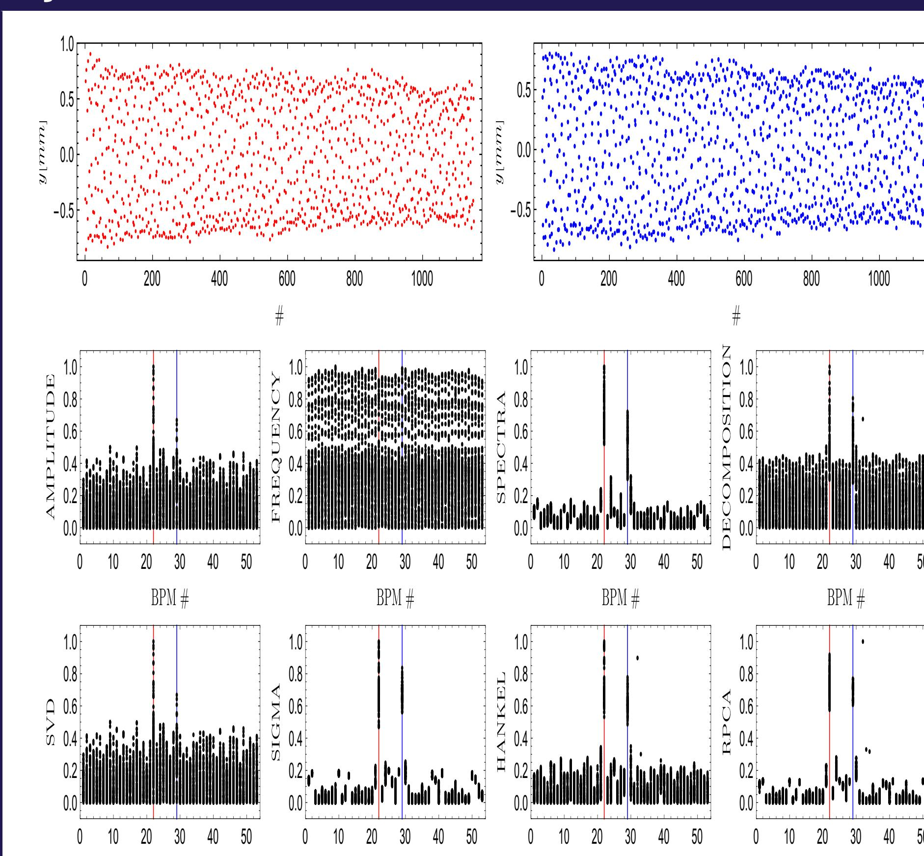
Fig. 7: Example of detected systematic anomalies from single measurement (top plots). Normalized features for all BPMs (bottom plots). Positions of signals with anomalies indicated with lines.
