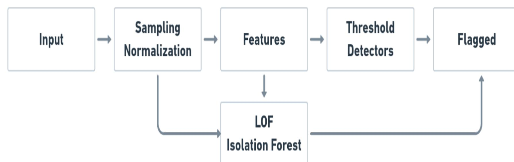
Fig. 2: Anomaly detection loop workflow.
