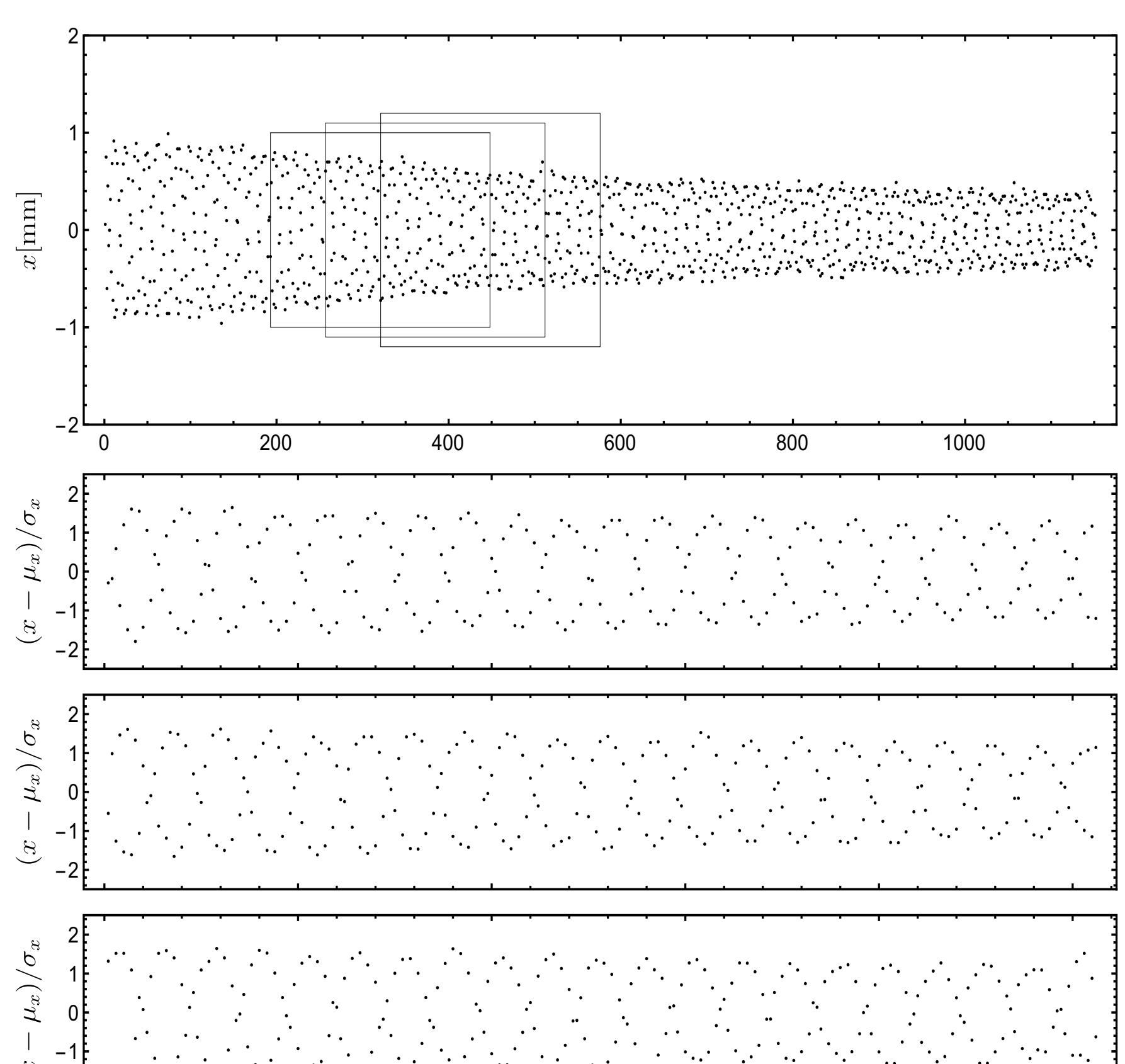
Fig. 3: Signal sampling. Each BPM signal is divided into smaller shifted samples.
