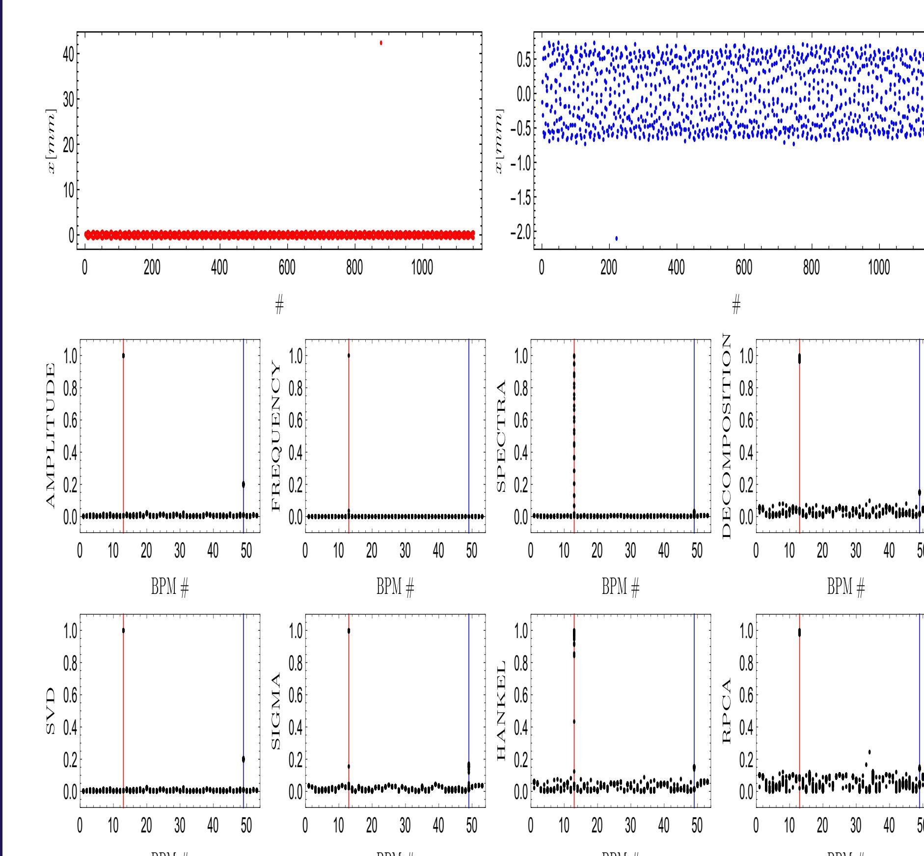
Fig. 6: Example of detected spike anomalies from single measurement (top plots). Normalized features for all BPMs (bottom plots). Positions of signals with anomalies indicated with lines.
