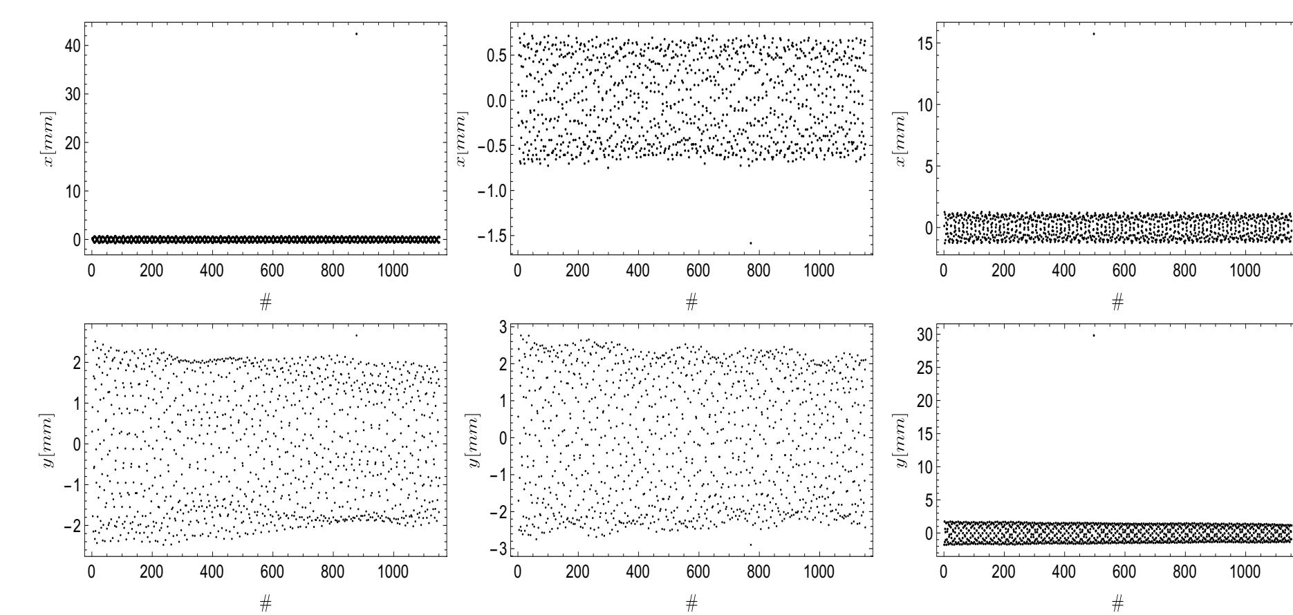
Fig. 1: Examples of spike anomalies in BPM signals at the VEPP-4M. Spike anomalies are correlated across planes.
