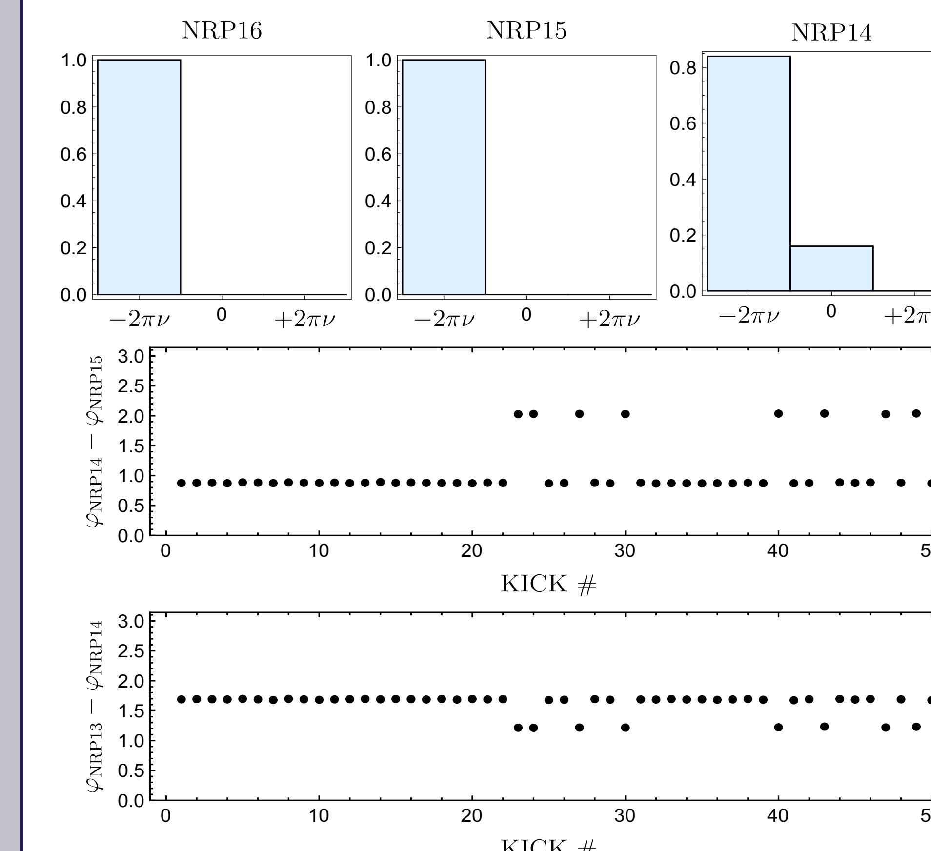
Fig. 9: BPM synchronization. Phase measurement requires synchronization of the first turn between BPMs. Measured phase advance can be compared with model to check the first turn synchronization.
