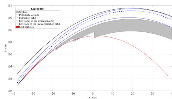
Figure 6: Graph of losses of ion beam <sup>209</sup>Bi<sup>38+</sup> in an electrostatic deflector with a constant gap
