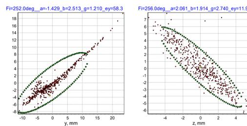
Figure 5: The horizontal and vertical beam emittances at the PMQ entrance (A/Z=5.5, B<sub>0</sub>=1.55 T)
