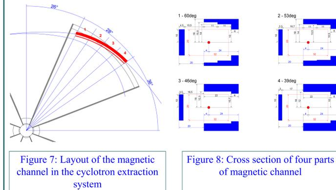
Figure 7: Layout of the magnetic channel in the cyclotron extraction system
