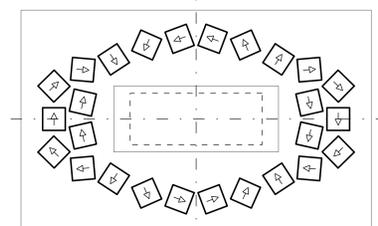
Figure 9: Cross section of PMQ consisting of 26 permanent magnets
