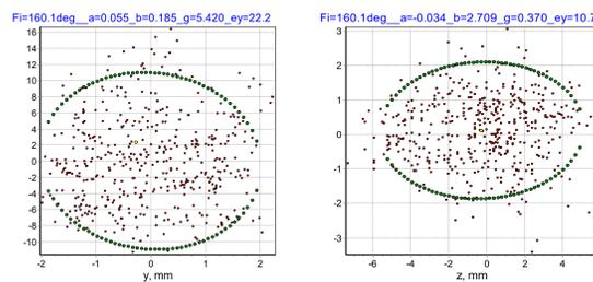
Figure 3: The horizontal and vertical beam emittances at the deflector entrance (A/Z=5.5, B<sub>0</sub>=1.55 T)
