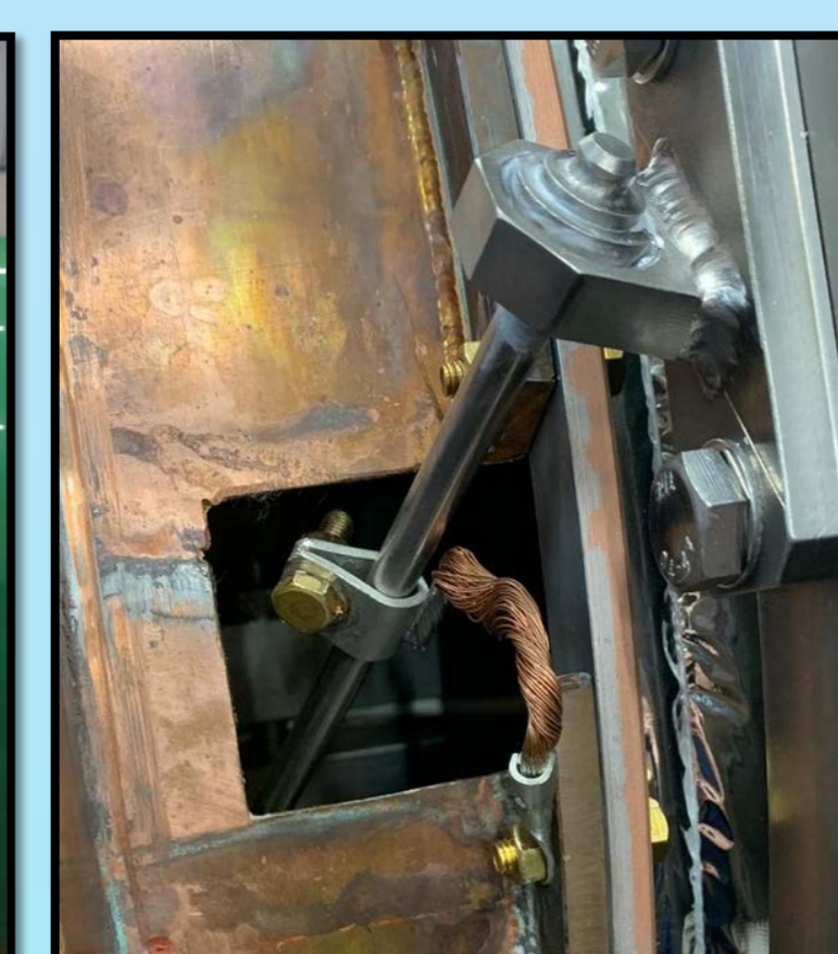
Technological hole in the thermal shield for the suspension system.
