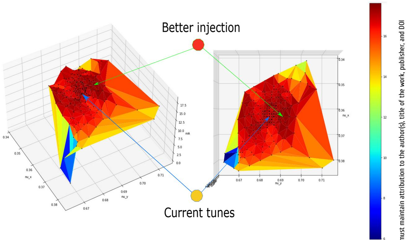
Figure 5: Amount of damping ring captured particles vs. tunes for "VEPP-2000 positron" IC mode.
